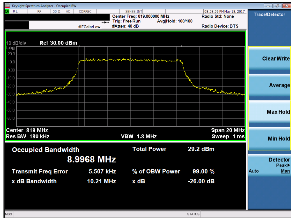
Plot 7-12. Occupied Bandwidth Plot (10MHz 64-QAM – RB Size 50)
