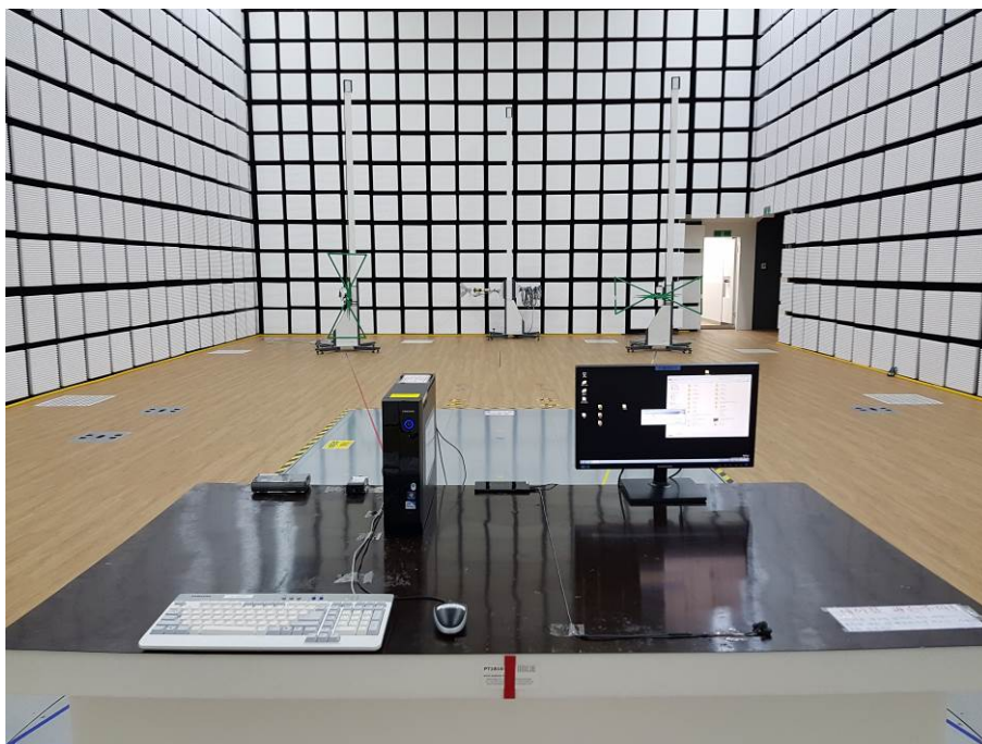
[ Radiated Disturbance for Below 1 GHz – Front ]
