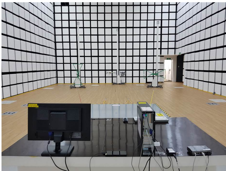
[ Radiated Disturbance for Below 1 GHz – Rear ]
