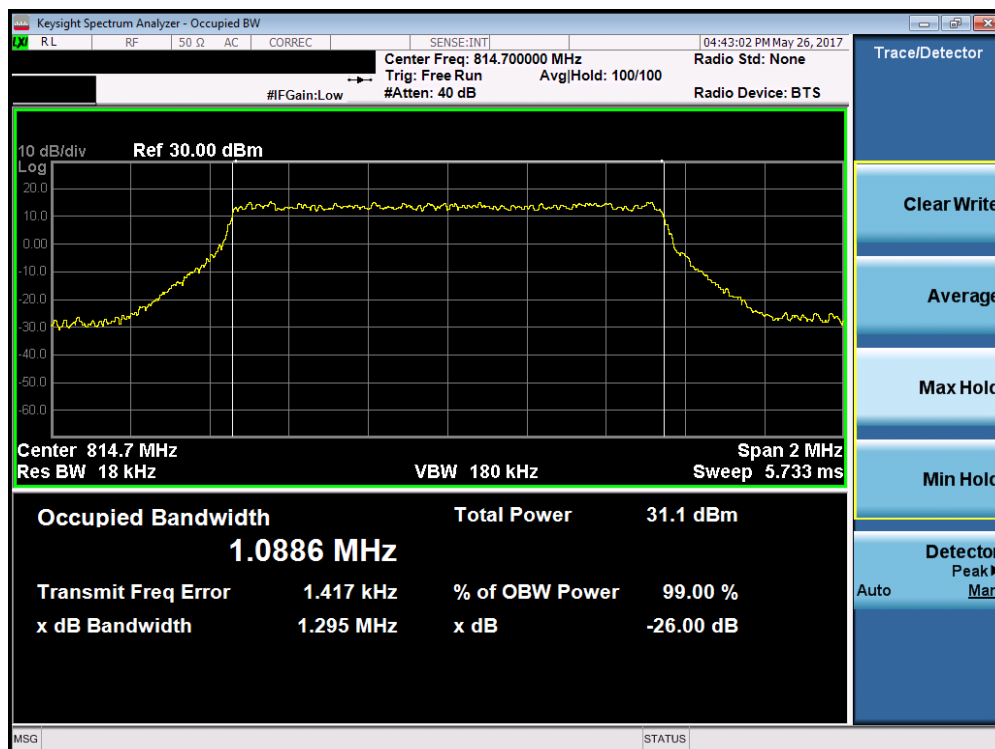
Plot 7-1. Occupied Bandwidth Plot (1.4MHz QPSK – RB Size 6– Low Channel)
