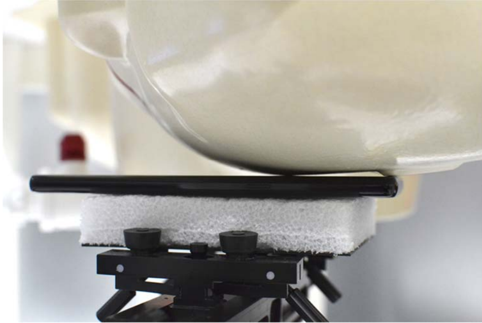
SAR Test Setup Photo 3 – Left Cheek
