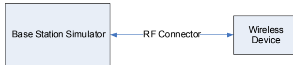
Figure 9-3 Power Measurement Setup
