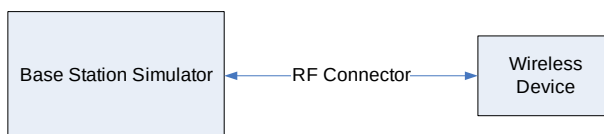
Figure 9-1 Power Measurement Setup
