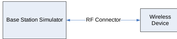
Figure 9-2 Power Measurement Setup
