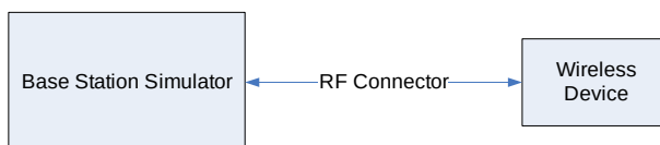
Figure 9-1 Power Measurement Setup
