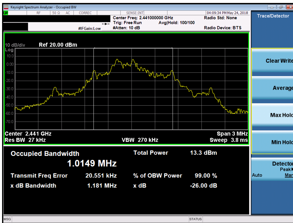
Plot 7-1. Occupied Bandwidth Plot (ANT+ – Ch. 39)
