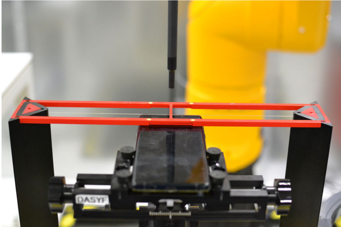
Figure 18-1 Ear Reference Point HAC Phantom Alignment
