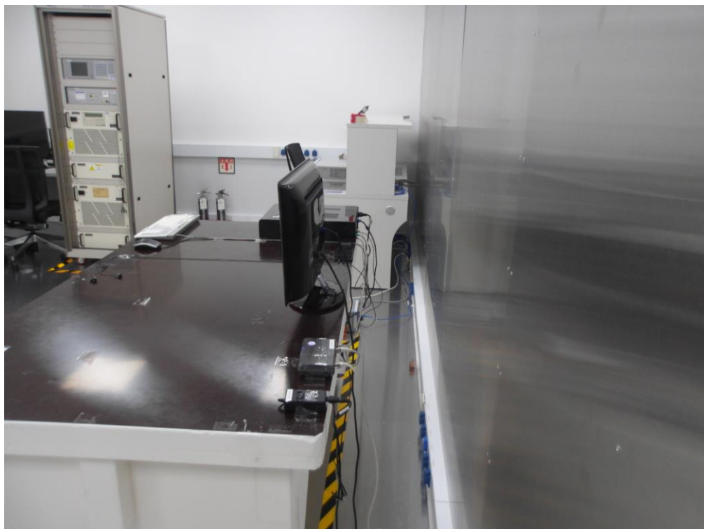
[ Conducted Disturbance – Rear ]
