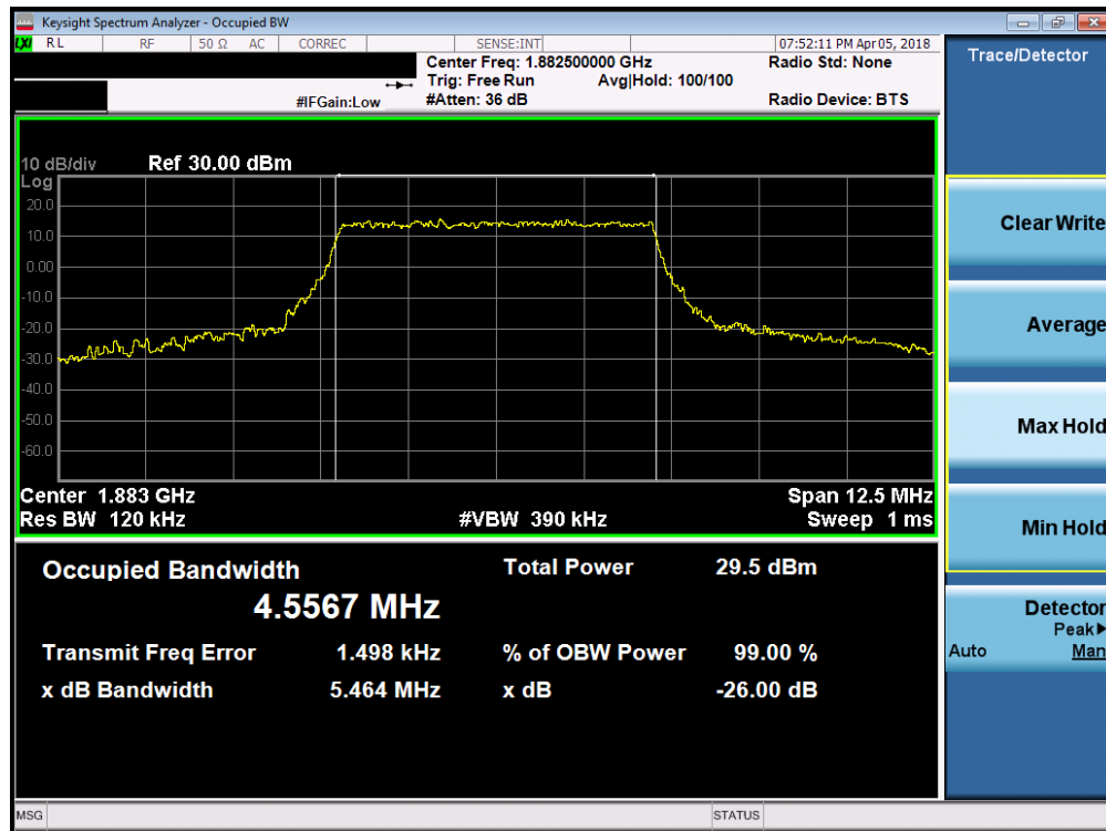
Plot 7-60. Occupied Bandwidth Plot (Band 25/2 - 5.0MHz 64-QAM - Full RB Configuration)
