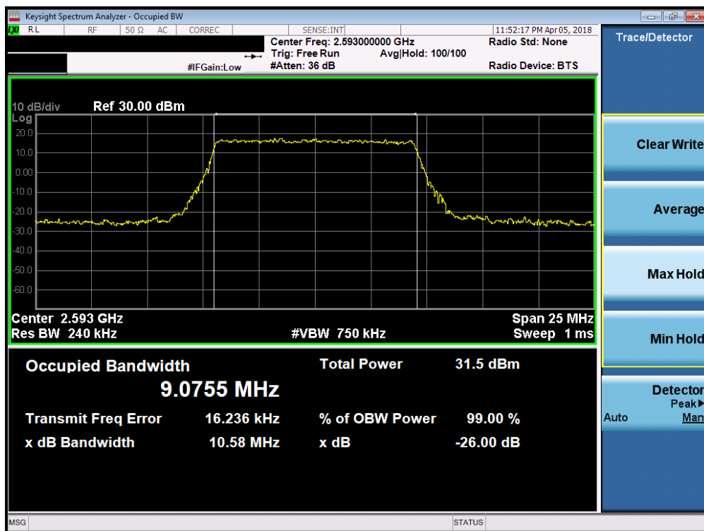
Plot 7-85. Occupied Bandwidth Plot (Band 41/38 - 10.0MHz QPSK - Full RB Configuration)
