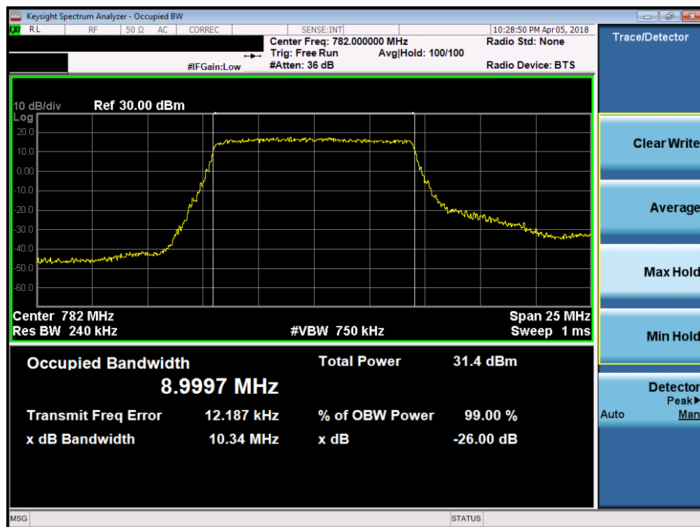
Plot 7-16. Occupied Bandwidth Plot (Band 13 - 10.0MHz QPSK - Full RB Configuration)
