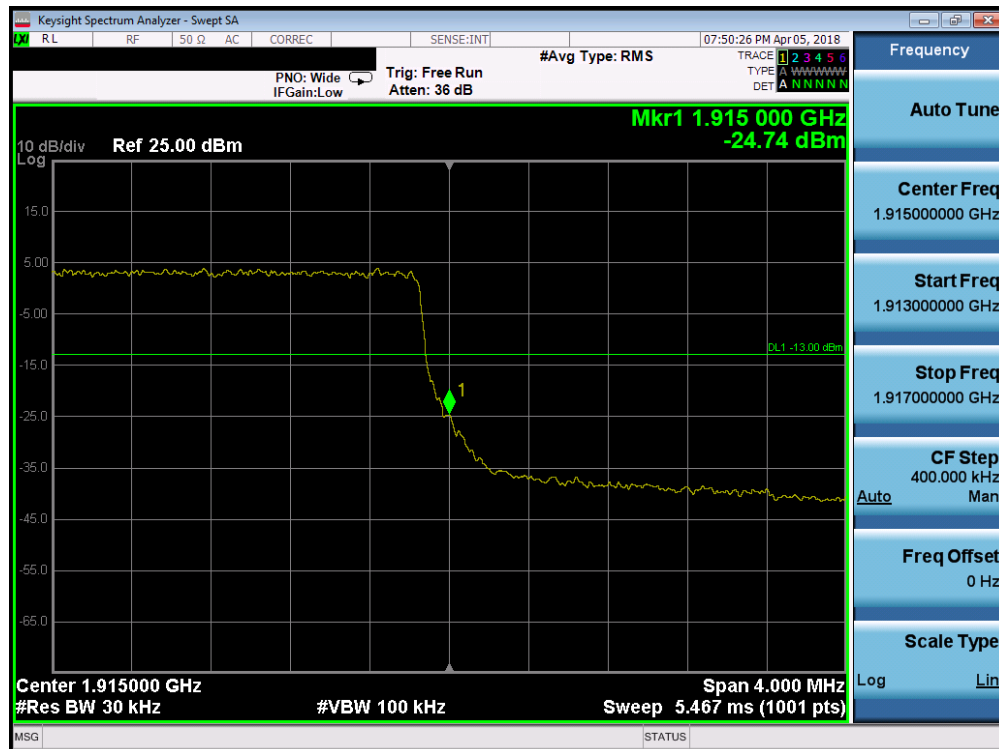
Plot 7-227. Upper Band Edge Plot (Band 25 - 3.0MHz QPSK - Full RB Configuration)
