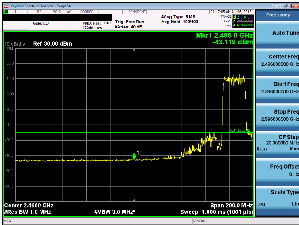
Plot 7-275. Lower ACP Plot (Band 38 - 20.0MHz QPSK - RB Size 25)
