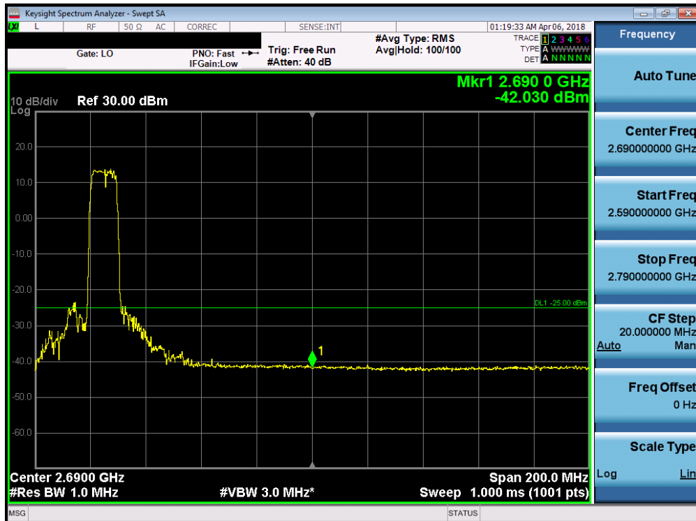
Plot 7-272. Upper ACP Plot (Band 38 - 10.0MHz QPSK - RB Size 25)
