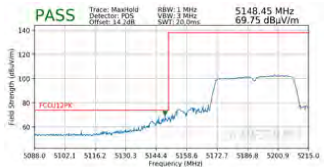
Plot 7-215. Radiated Lower Band Edge Plot (Peak – UNII Band 1)
