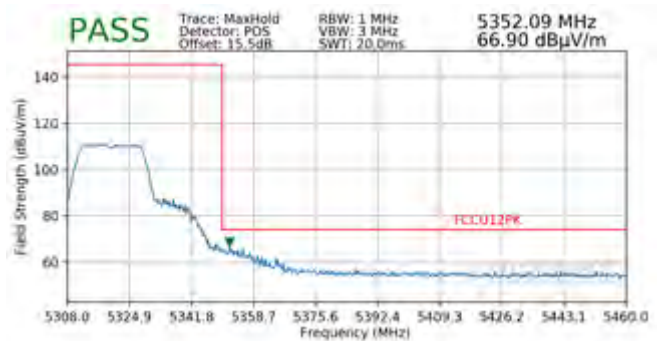
Plot 7-240. Radiated Band Edge Plot (Peak – WCP)
