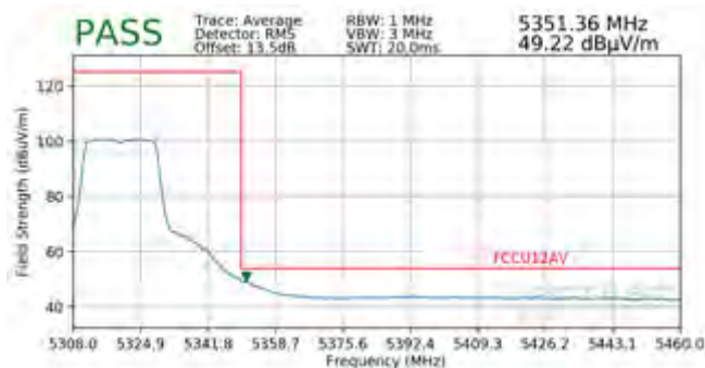
Plot 7-180. Radiated Upper Band Edge Plot (Average – UNII Band 2A)
