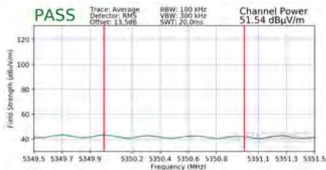
Plot 7-216. Radiated Upper Band Edge Plot (Average – UNII Band 2A)
