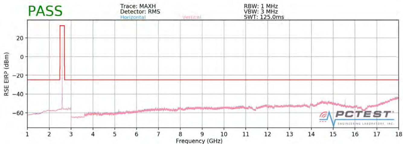
Plot 7-271. Radiated Spurious Plot 1GHz - 18GHz (Band 41)
