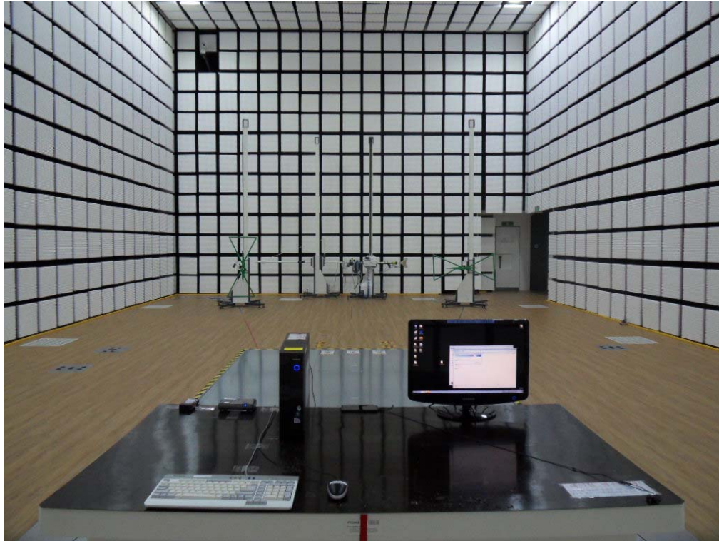
[ Radiated Disturbance for Below 1 GHz – Front ]
