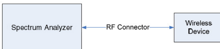
Figure 7-1. Test Instrument & Measurement Setup
