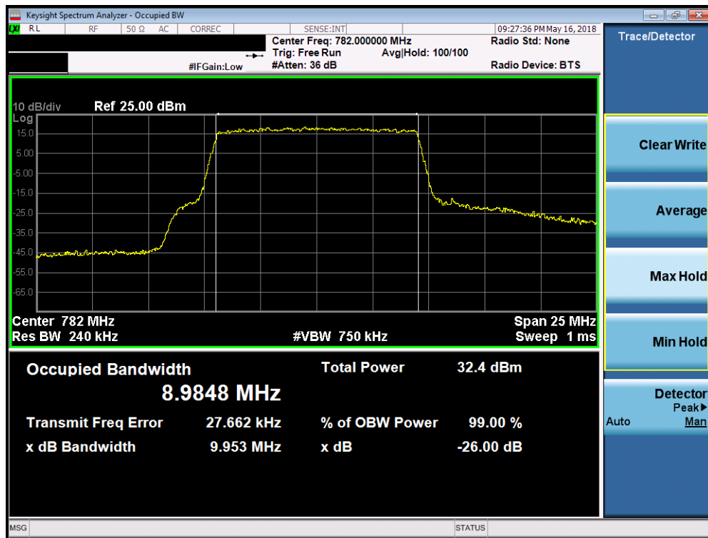
Plot 7-28. Occupied Bandwidth Plot (Band 13 - 10.0MHz QPSK - Full RB Configuration)
