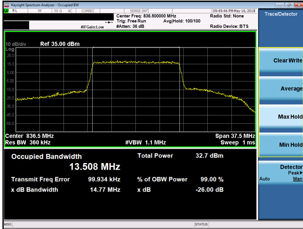
Plot 7-43. Occupied Bandwidth Plot (Band 26 - 15.0MHz QPSK - Full RB Configuration)
