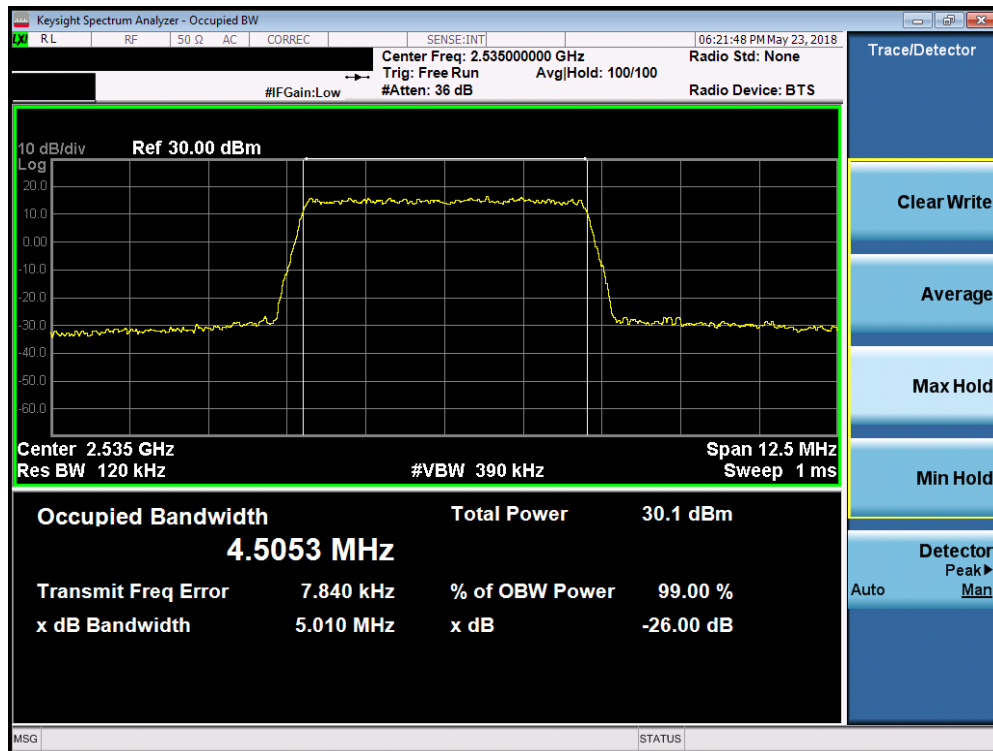
Plot 7-95. Occupied Bandwidth Plot (Band 7 - 5.0MHz 16-QAM - Full RB Configuration)
