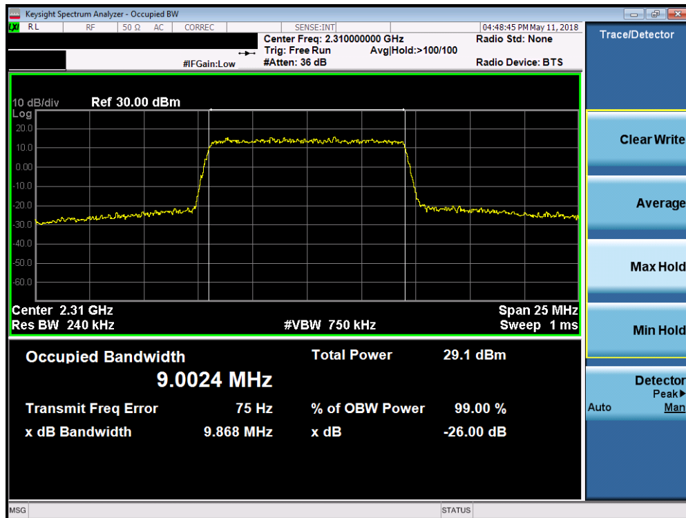
Plot 7-87. Occupied Bandwidth Plot (Band 30 - 10.0MHz 64-QAM - Full RB Configuration)
