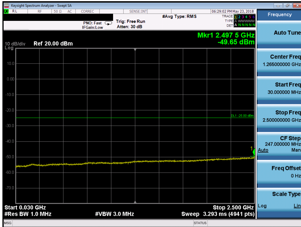
Plot 7-208. Conducted Spurious Plot (Band 7 - 15.0MHz QPSK - RB Size 1, RB Offset 0 - High Channel)
