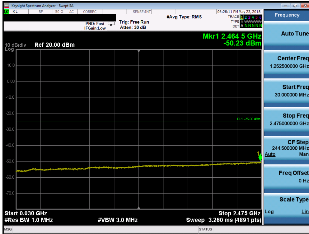
Plot 7-202. Conducted Spurious Plot (Band 7 - 15.0MHz QPSK - RB Size 1, RB Offset 0 - Low Channel)
