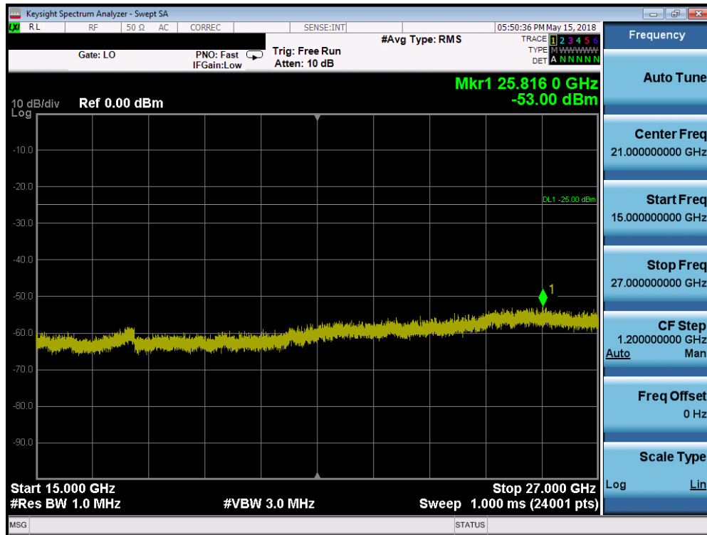
Plot 7-231. Conducted Spurious Plot (Band 41 - 20.0MHz QPSK - RB Size 1, RB Offset 0 - Low Channel)
