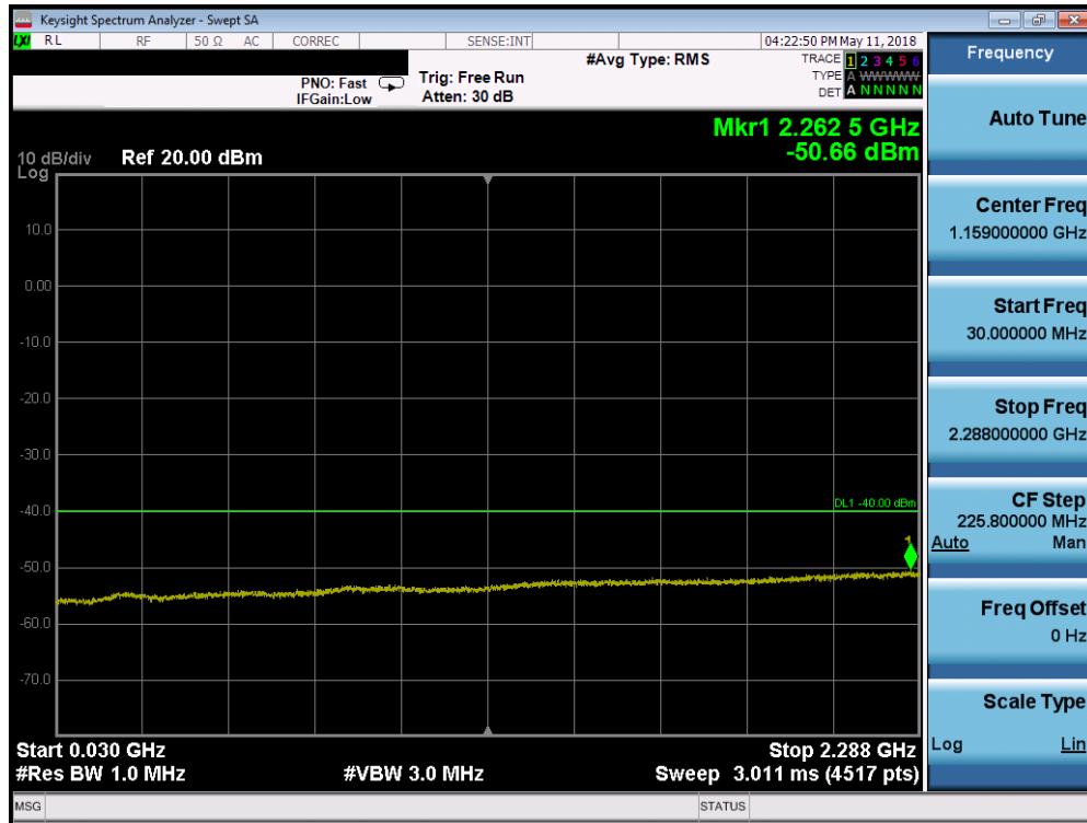
Plot 7-193. Conducted Spurious Plot (Band 30 - 5.0MHz QPSK - RB Size 1, RB Offset 0 - Low Channel)
