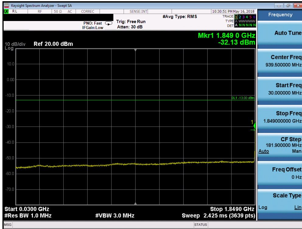
Plot 7-181. Conducted Spurious Plot (Band 25/2 - 20.0MHz QPSK - RB Size 1, RB Offset 0 - Low Channel)
