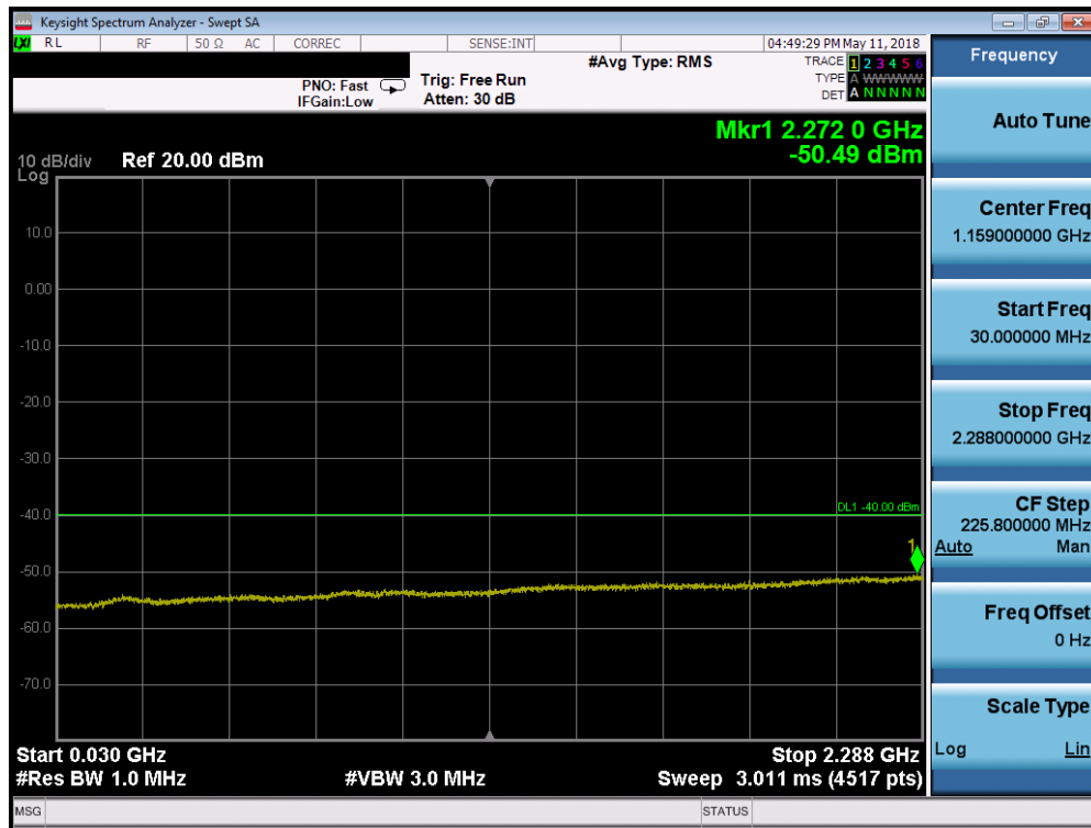
Plot 7-190. Conducted Spurious Plot (Band 30 - 10.0MHz QPSK - RB Size 1, RB Offset 0 - Mid Channel)
