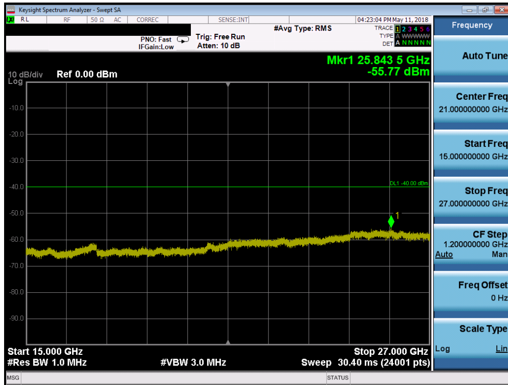
Plot 7-195. Conducted Spurious Plot (Band 30 - 5.0MHz QPSK - RB Size 1, RB Offset 0 - Low Channel)
