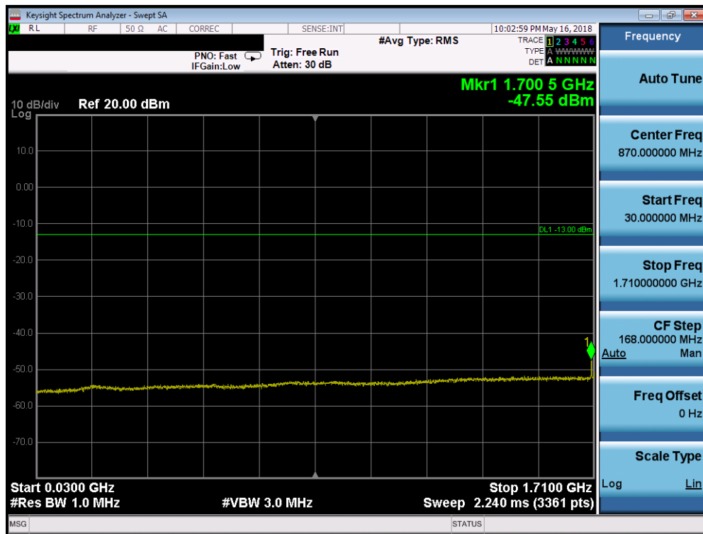
Plot 7-175. Conducted Spurious Plot (Band 66/4 - 20.0MHz QPSK - RB Size 1, RB Offset 0 - Mid Channel)
