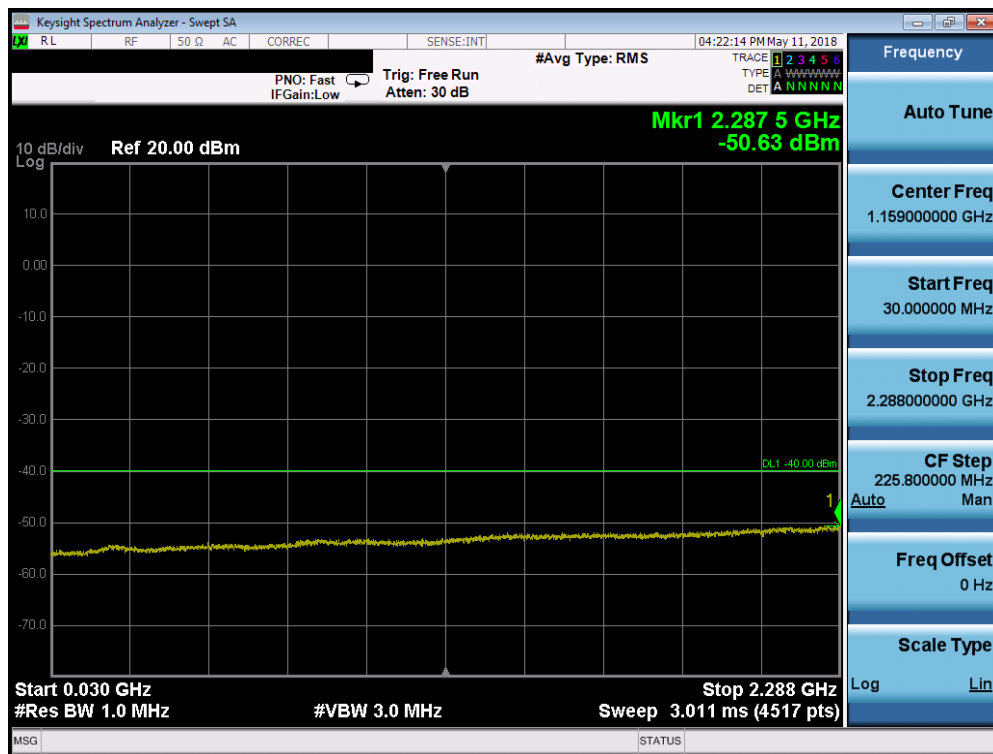
Plot 7-196. Conducted Spurious Plot (Band 30 - 5.0MHz QPSK - RB Size 1, RB Offset 0 - Mid Channel)
