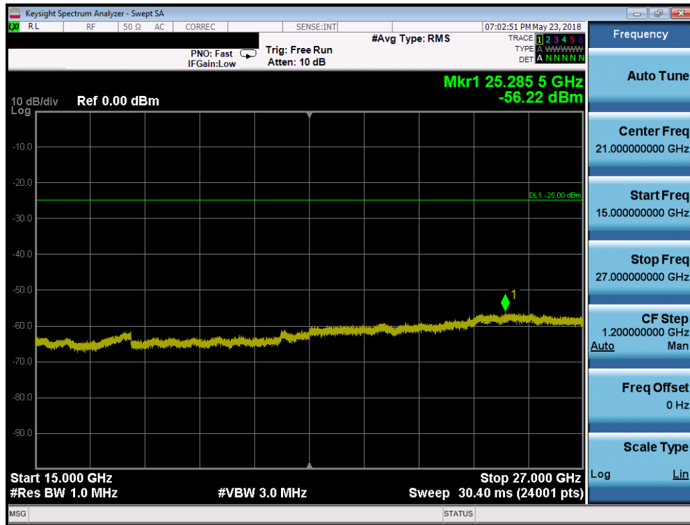
Plot 7-213. Conducted Spurious Plot (Band 7 - 15.0MHz QPSK - RB Size 1, RB Offset 0 - Low Channel)
