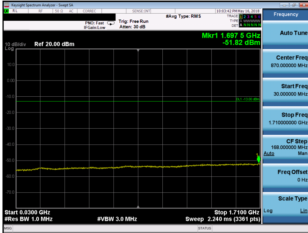
Plot 7-178. Conducted Spurious Plot (Band 66/4 - 20.0MHz QPSK - RB Size 1, RB Offset 0 - High Channel)
