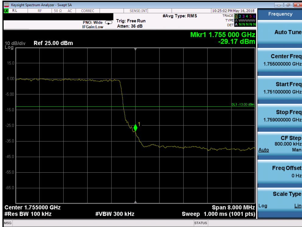
Plot 7-290. Upper Band Edge Plot (Band 4 - 10.0MHz QPSK - Full RB Configuration)
