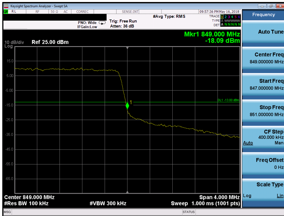
Plot 7-263. Upper Band Edge Plot (Band 26/5 - 3.0MHz QPSK - Full RB Configuration)
