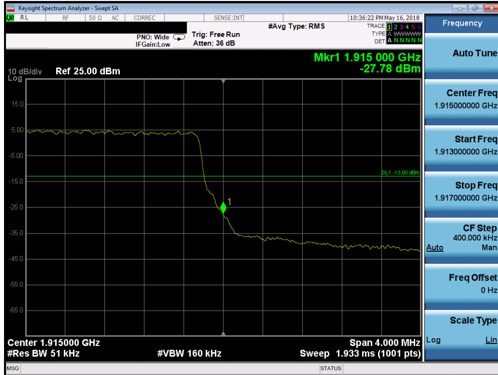
Plot 7-322. Upper Band Edge Plot (Band 25 - 5.0MHz QPSK - Full RB Configuration)
