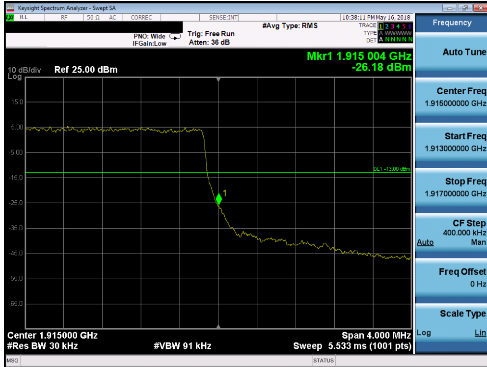
Plot 7-316. Upper Band Edge Plot (Band 25 - 3.0MHz QPSK - Full RB Configuration)
