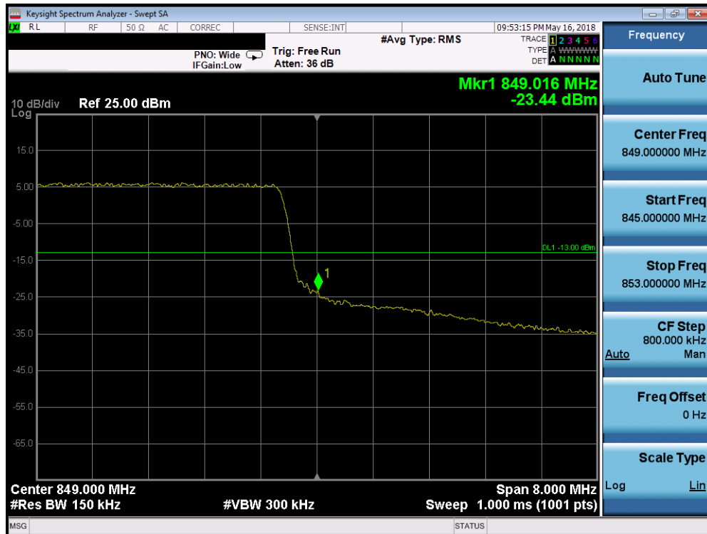
Plot 7-267. Upper Band Edge Plot (Band 26/5 - 10.0MHz QPSK - Full RB Configuration)
