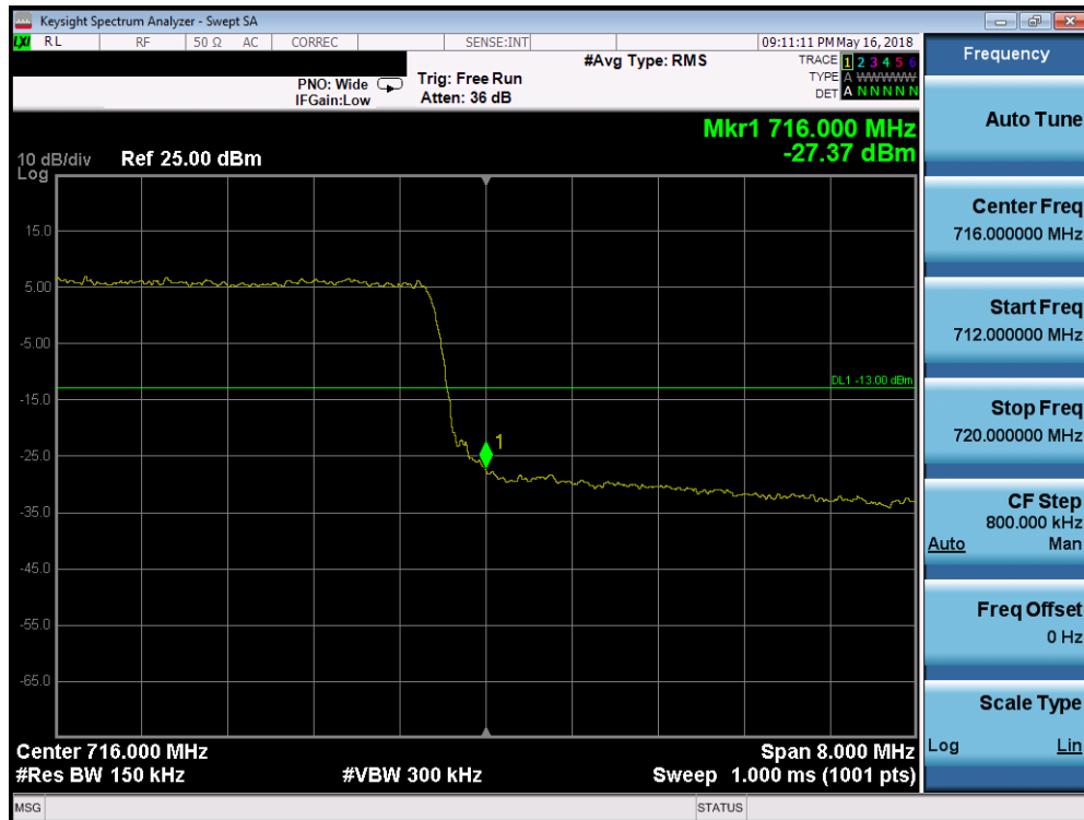
Plot 7-255. Upper Band Edge Plot (Band 12/17 - 10.0MHz QPSK - Full RB Configuration)
