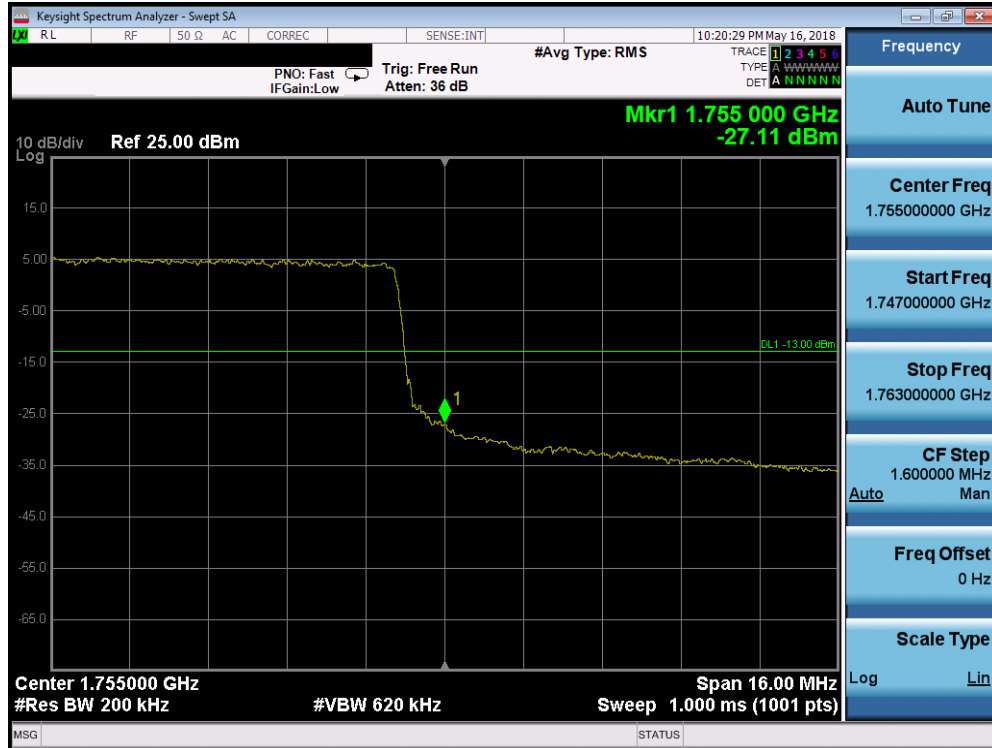
Plot 7-302. Upper Band Edge Plot (Band 4 - 20.0MHz QPSK - Full RB Configuration)
