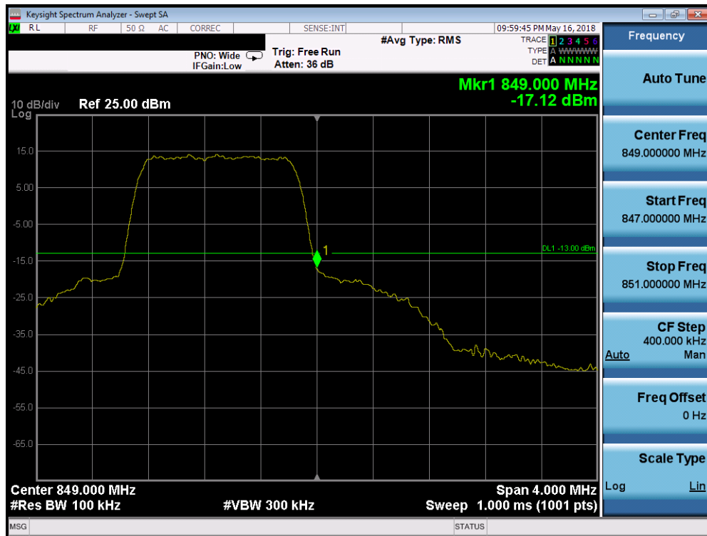
Plot 7-261. Upper Band Edge Plot (Band 26/5 - 1.4MHz QPSK - Full RB Configuration)
