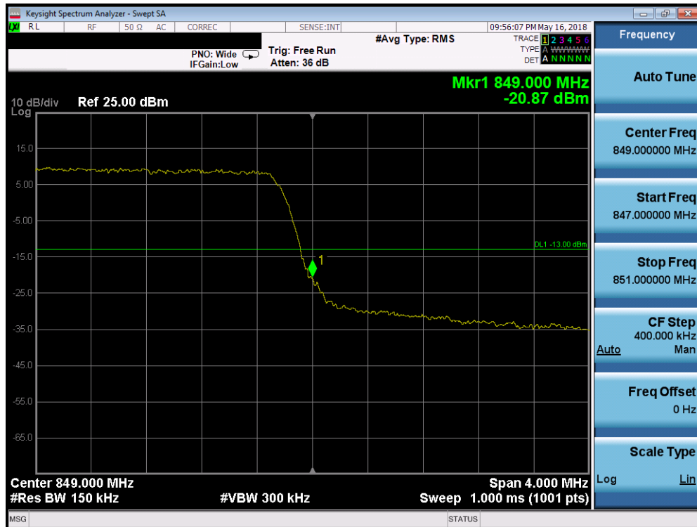
Plot 7-265. Upper Band Edge Plot (Band 26/5 - 5.0MHz QPSK - Full RB Configuration)
