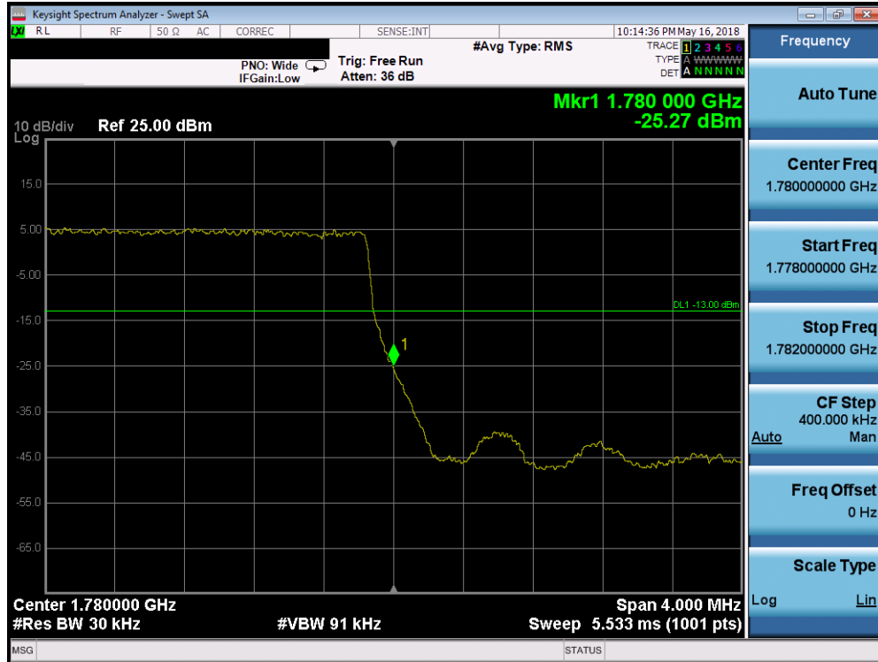
Plot 7-280. Upper Band Edge Plot (Band 66 - 3.0MHz QPSK - Full RB Configuration)
