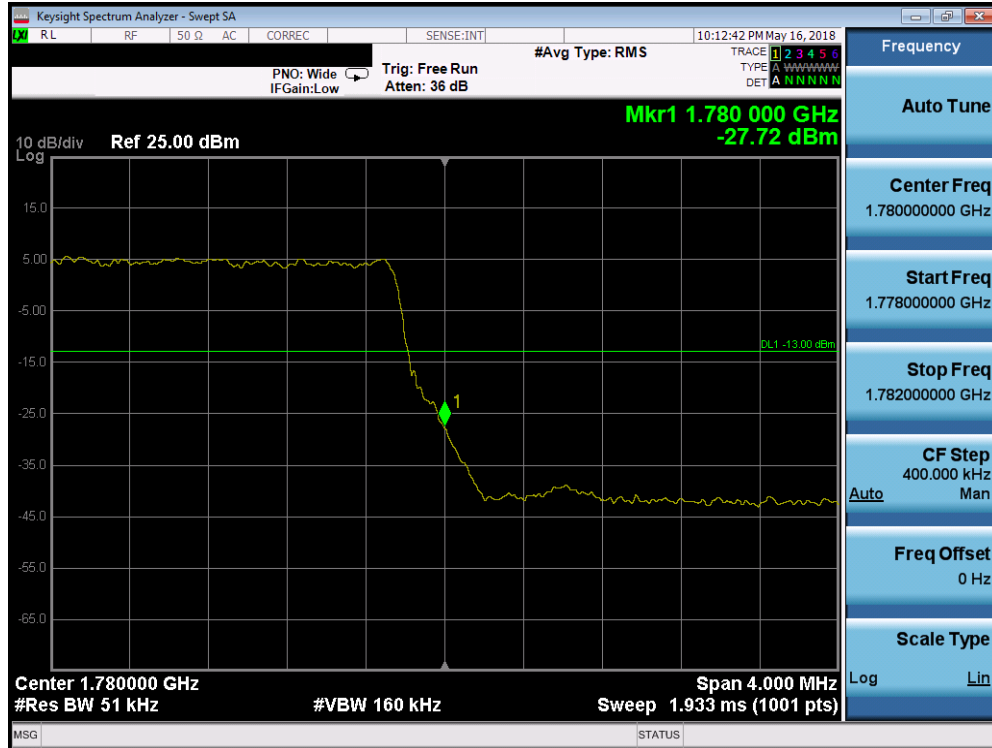
Plot 7-286. Upper Band Edge Plot (Band 66 - 5.0MHz QPSK - Full RB Configuration)
