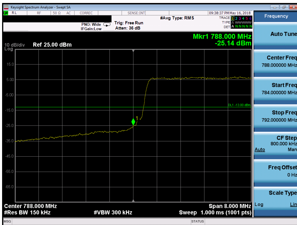
Plot 7-42. Lower Band Edge Plot (LTE Band 14 – 10MHz QPSK – Full RB Configuration)
