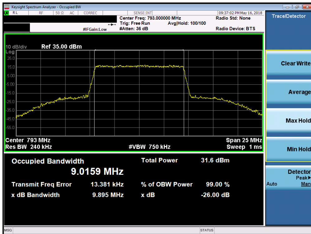
Plot 7-7. Occupied Bandwidth Plot (LTE Band 14 – 10MHz 16QAM – Full RB Configuration)
