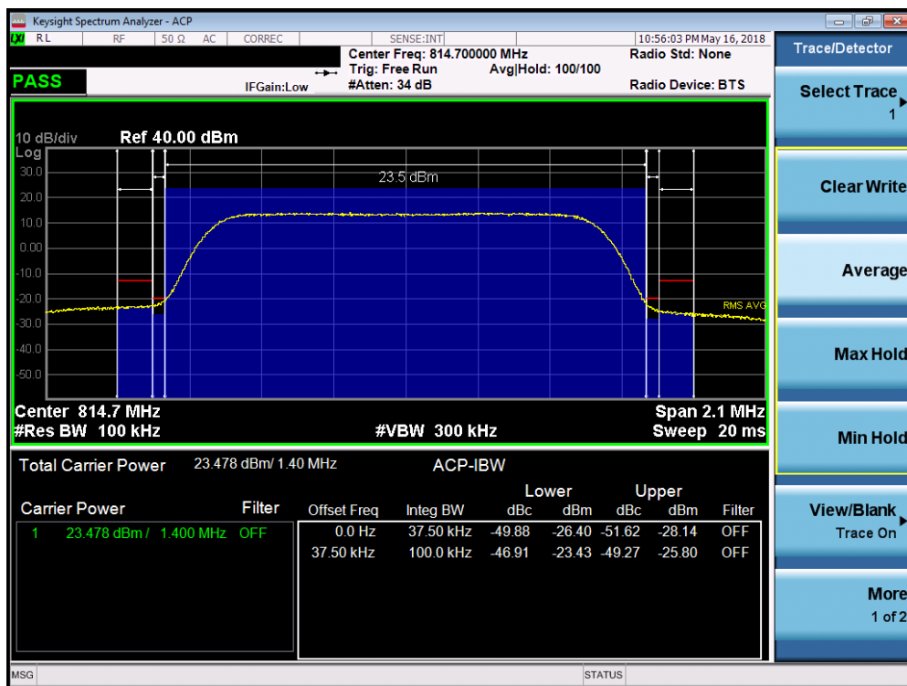
Plot 7-46. Channel Edge Plot (LTE Band 26 – 1.4MHz QPSK – RB Size 6– Low Channel)
