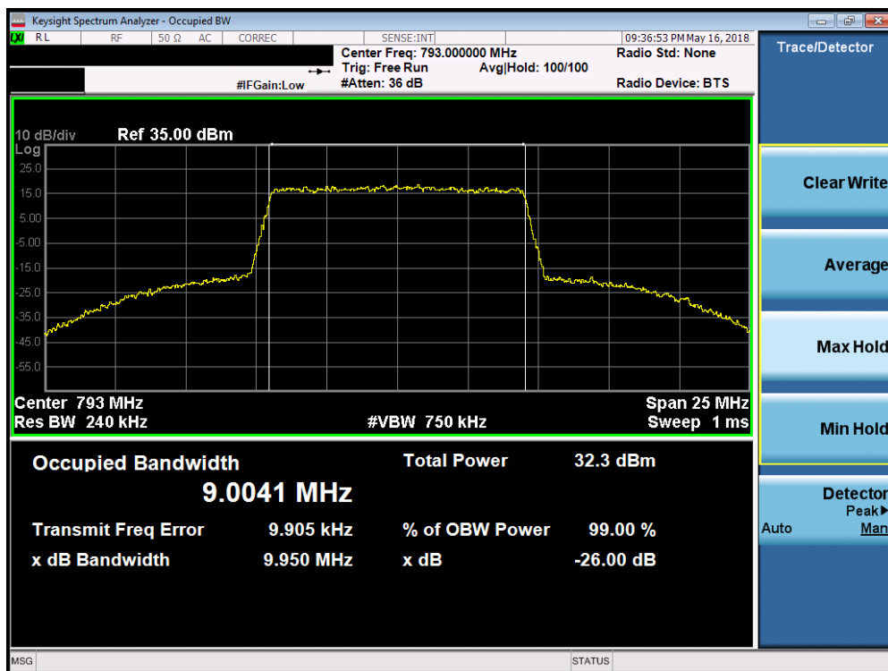
Plot 7-6. Occupied Bandwidth Plot (LTE Band 14 – 10MHz QPSK – Full RB Configuration)
