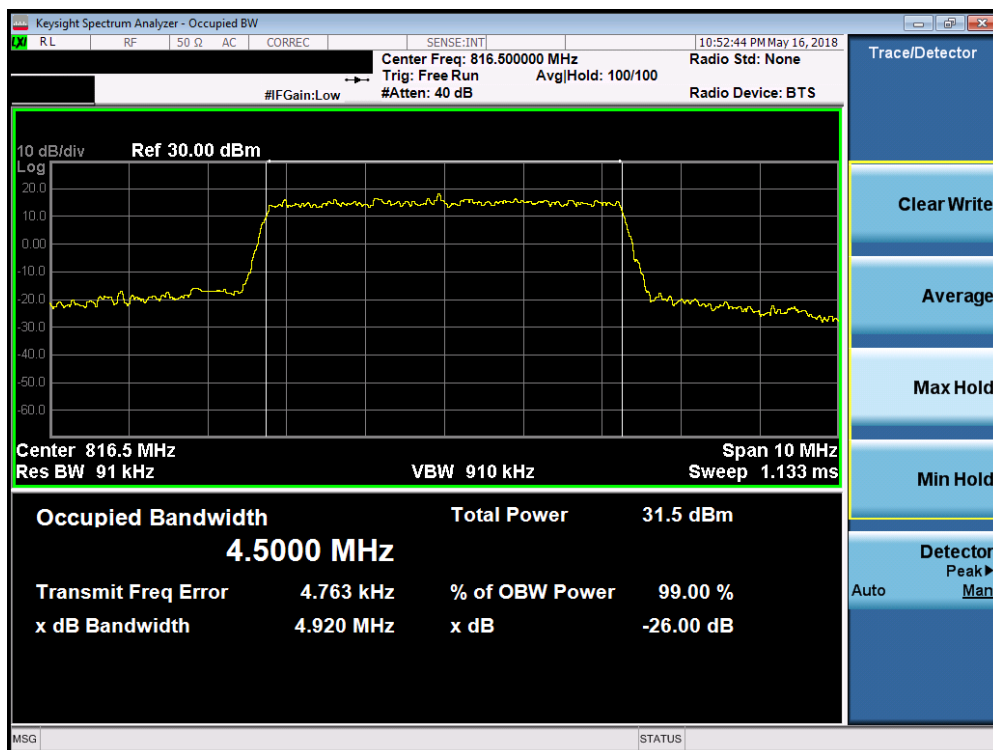
Plot 7-16. Occupied Bandwidth Plot (LTE B26 – 5MHz 16-QAM – RB Size 25– Low Channel)
