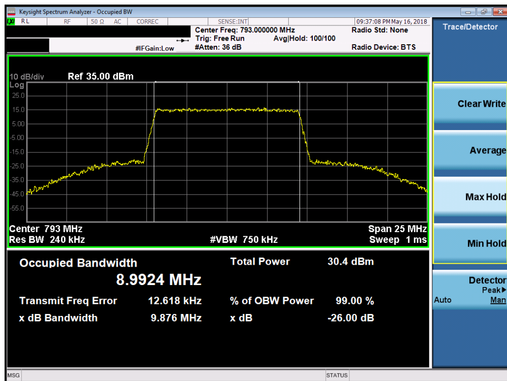
Plot 7-8. Occupied Bandwidth Plot (LTE Band 14 – 10MHz 64QAM – Full RB Configuration)
