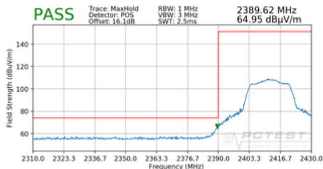
Plot 7-92. Radiated Restricted Band Edge Measurement MIMO with WCP (Peak)
