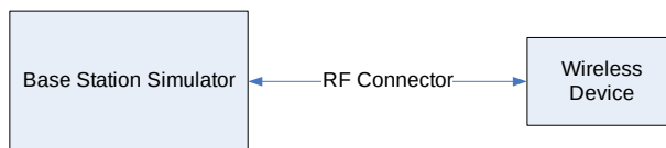
Figure 9-4 Power Measurement Setup
