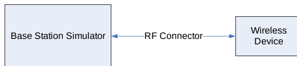
Figure 9-1 Power Measurement Setup
