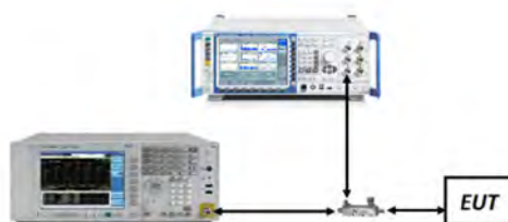
Figure 7-1. Test Instrument & Measurement Setup
