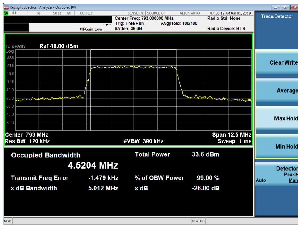
Plot 7-23. Occupied Bandwidth Plot (LTE Band 14, 5MHz QPSK – RB Size 25)
