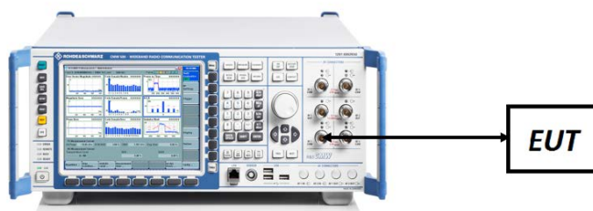
Figure 7-4. ERP/EIRP Measurement Setup
