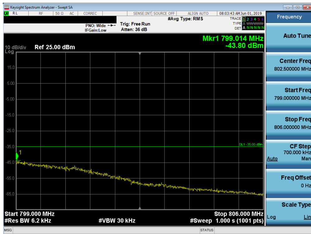
Plot 7-56. Upper Emission Mask Plot (LTE Band 14, 5MHz QPSK - RB Size 25)
