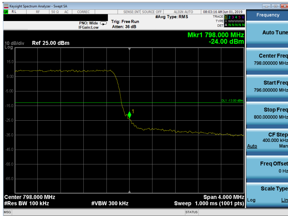
Plot 7-55. Upper Band Edge Plot (LTE Band 14, 5MHz QPSK - RB Size 25)
