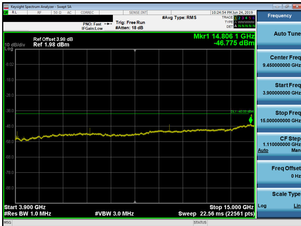
Plot 7-31. Conducted Spurious Plot (Band 48 - 20.0MHz QPSK - RB Size 1, RB Offset 99 - High Channel)
