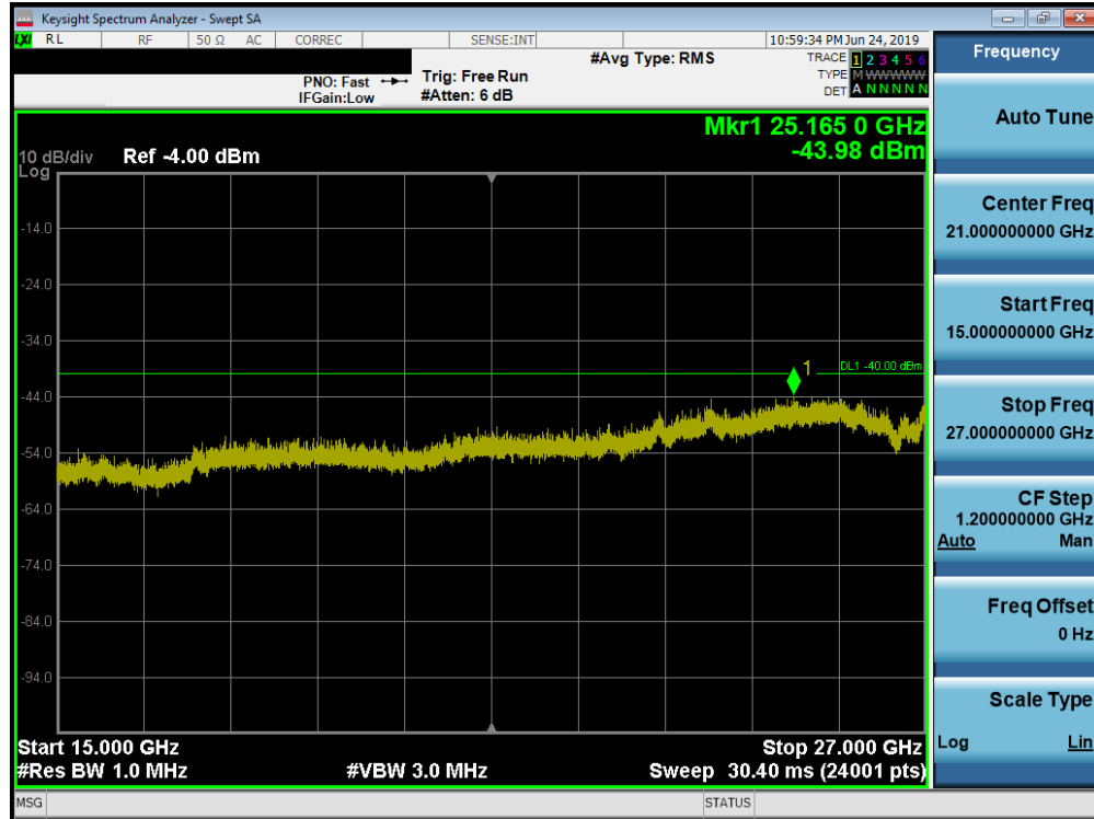
Plot 7-32. Conducted Spurious Plot (Band 48 - 20.0MHz QPSK - RB Size 1, RB Offset 99 - High Channel)
