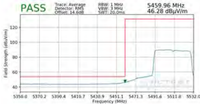
Plot 7-339. Radiated Lower Band Edge Plot SISO ANT2 (Average – UNII Band 2C – 484 Tones)
