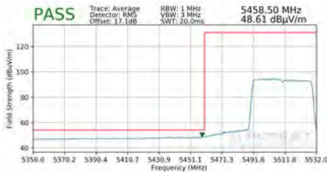
Plot 7-318. Radiated Lower Band Edge Plot SISO ANT1 (Average – UNII Band 2C – 484 Tones)
