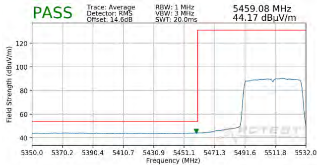
Plot 7-360. Radiated Lower Band Edge Plot MIMO (Average - UNII Band 2C - 484 Tones)
