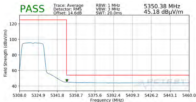
Plot 7-351. Radiated Upper Band Edge Plot MIMO (Average – UNII Band 2A – 242 Tones)
