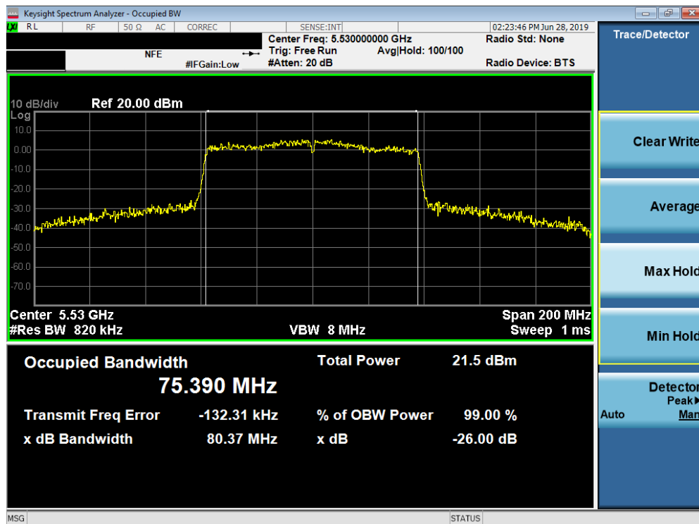
Plot 7-91. 26dB Bandwidth Plot SISO ANT2 (80MHz BW 802.11ac (UNII Band 2C) – Ch. 106)
