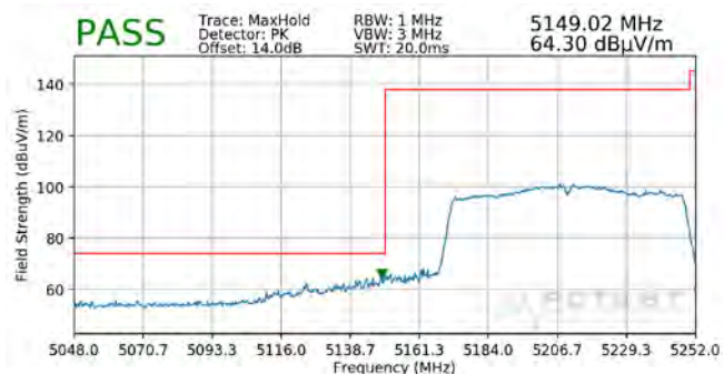
Plot 7-348. Radiated Lower Band Edge Plot MIMO (Peak – UNII Band 1)
