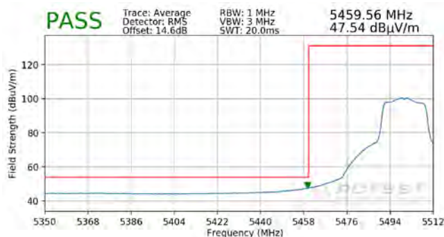
Plot 7-333. Radiated Lower Band Edge Plot MIMO (Average – UNII Band 2C)
