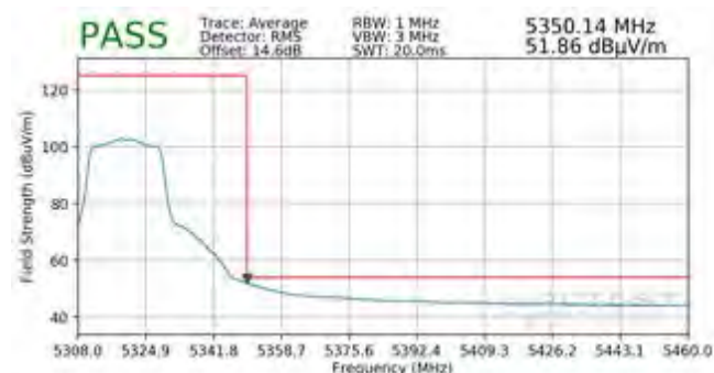
Plot 7-282. Radiated Upper Band Edge Plot SISO ANT1 (Average – UNII Band 2A)
