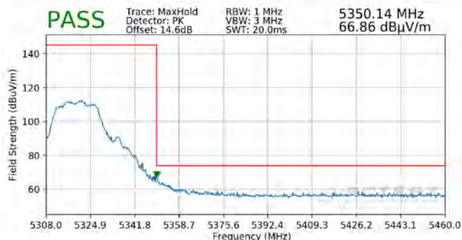
Plot 7-325. Radiated Upper Band Edge Plot MIMO (Peak – UNII Band 2A)
