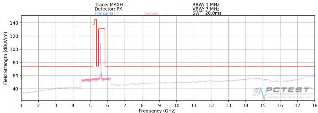
Plot 7-267. Radiated Spurious Plot above 1GHz SISO ANT2 (802.11a – U2C Ch. 120)
