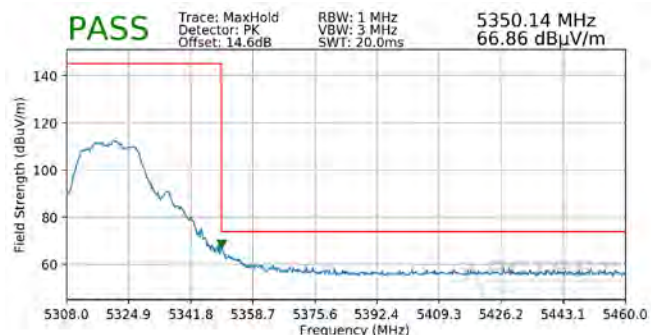
Plot 7-332. Radiated Upper Band Edge Plot MIMO (Peak – UNII Band 2A)
