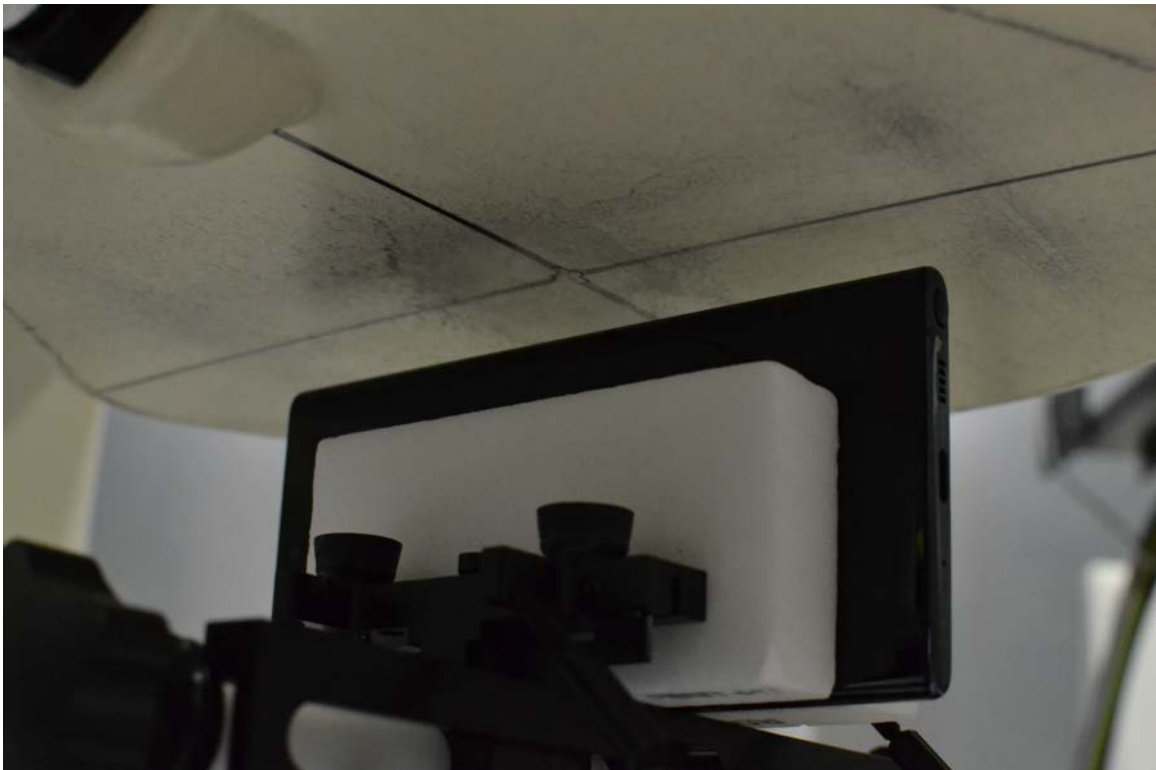
SAR Test Setup Photo 16 – Right Side at 10 mm
