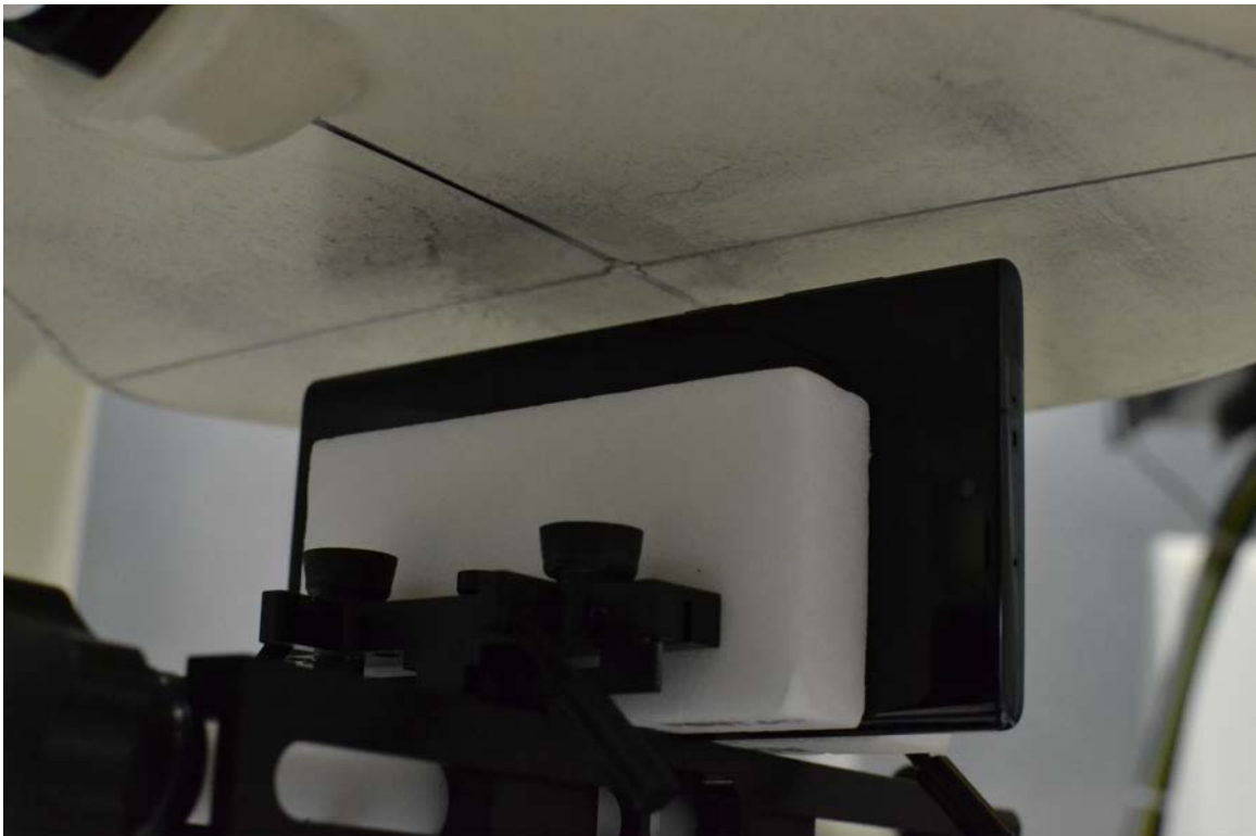
SAR Test Setup Photo 18 – Left Side at 10 mm
