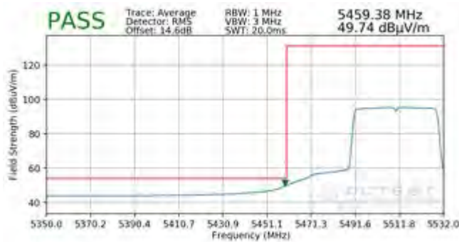
Plot 7-372. Radiated Lower Band Edge Plot SISO ANT1 (Average – UNII Band 2C – 484 Tones)
