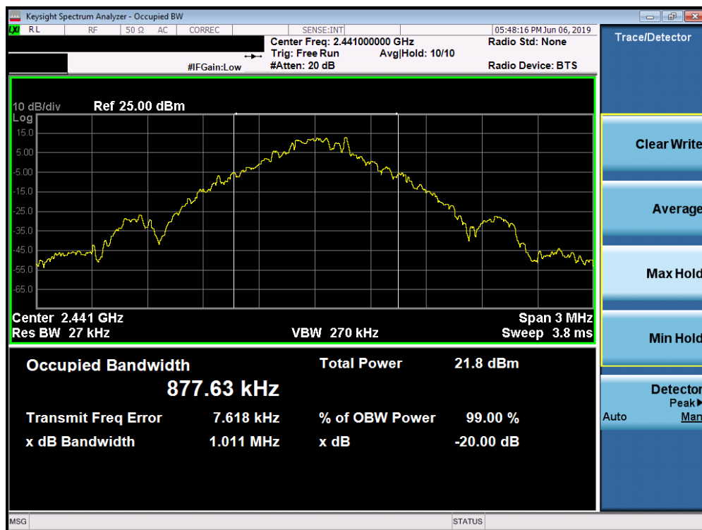
Plot 7-2. 20dB Bandwidth Plot (Bluetooth, 1Mbps – Ch. 39)
