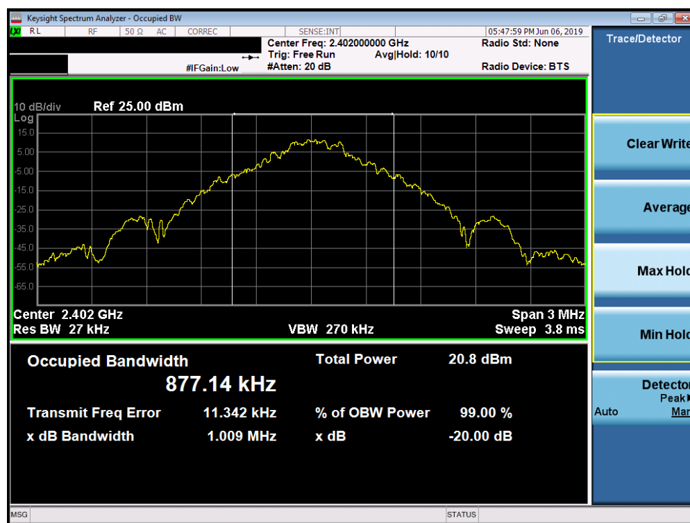
Plot 7-1. 20dB Bandwidth Plot (Bluetooth, 1Mbps – Ch. 0)
