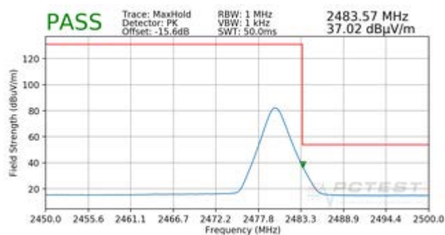
Plot 7-46. Radiated Restricted Upper Band Edge Measurement (Average)
