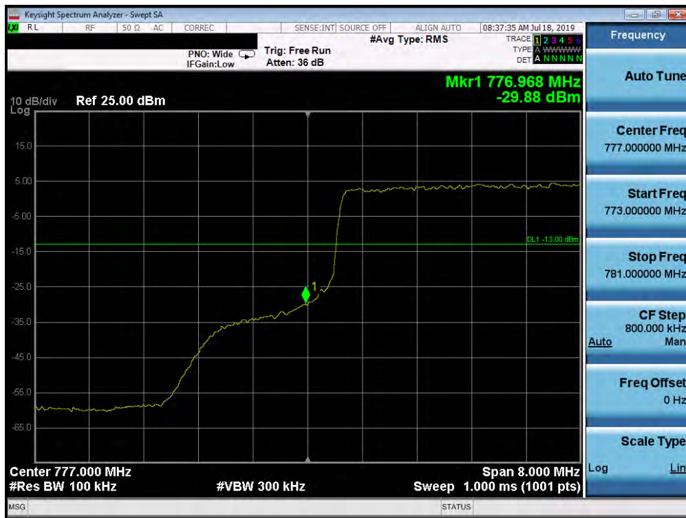
Plot 7-112. Lower Band Edge Plot (Band 13 - 10.0MHz QPSK - Full RB Configuration)
