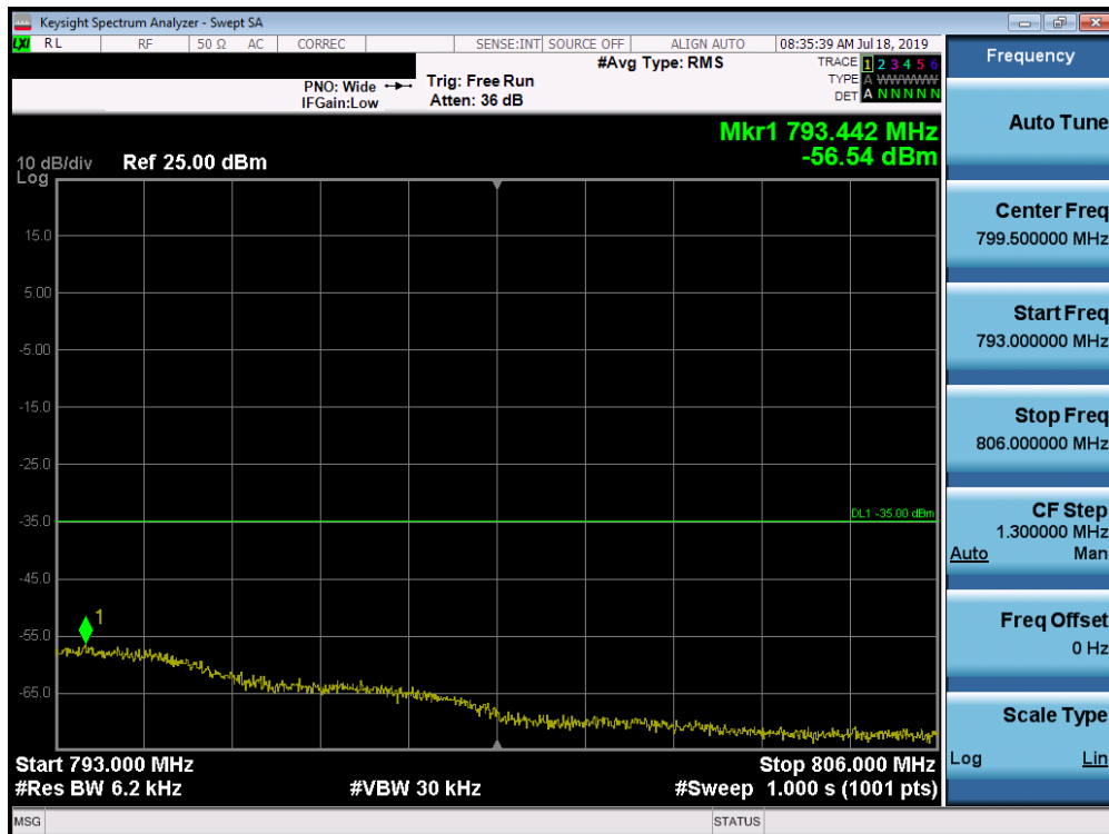
Plot 7-111. Upper Emission Mask Plot (Band 13 - 5.0MHz QPSK - Full RB Configuration)
