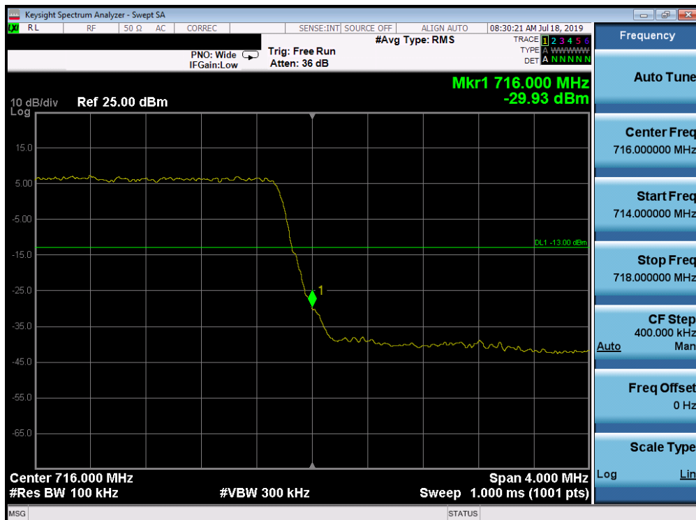
Plot 7-105. Upper Band Edge Plot (Band 12 - 5.0MHz QPSK - Full RB Configuration)
