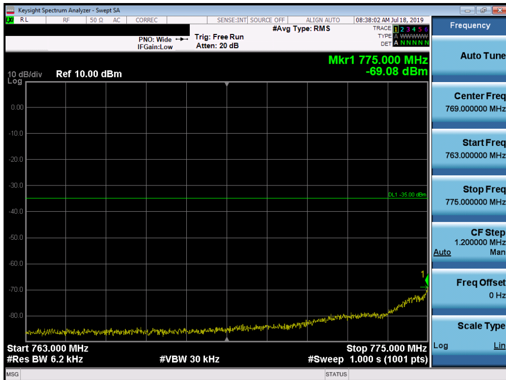
Plot 7-113. Lower Emission Mask Plot (Band 13 - 10.0MHz QPSK - Full RB Configuration)
