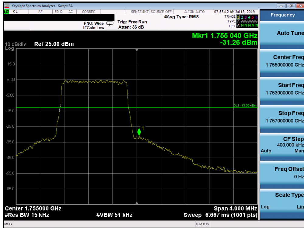
Plot 7-126. Upper Band Edge Plot (Band 4 - 1.4MHz QPSK - Full RB Configuration)
