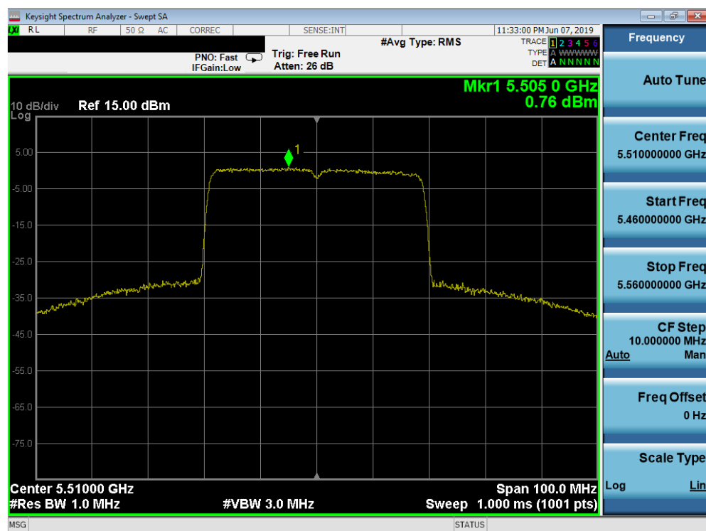
Plot 7-241. Power Spectral Density Plot SISO ANT2 (40MHz BW 802.11ax (UNII Band 2C) – Ch. 102)
