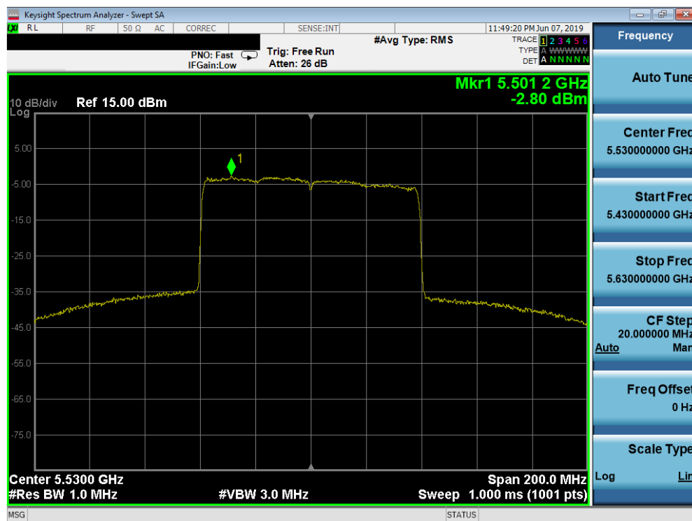
Plot 7-247. Power Spectral Density Plot SISO ANT2 (80MHz BW 802.11ax (UNII Band 2C) – Ch. 106)
