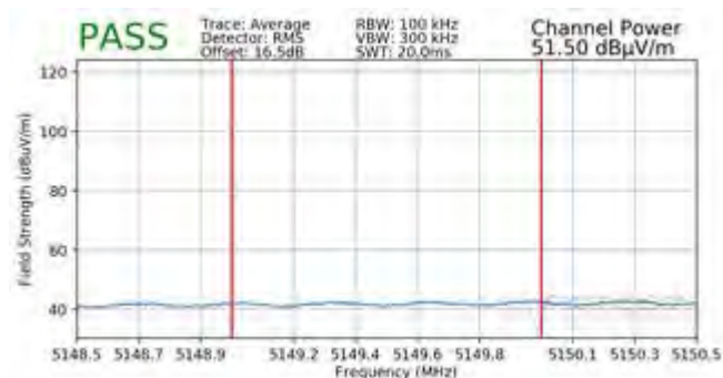
Plot 7-286. Radiated Lower Band Edge Plot SISO ANT1 (Average - UNII Band 1)
