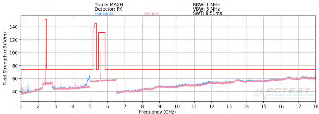
Plot 7-277. Radiated Spurious Plot above 1GHz (2.4GHz – 5GHz)
