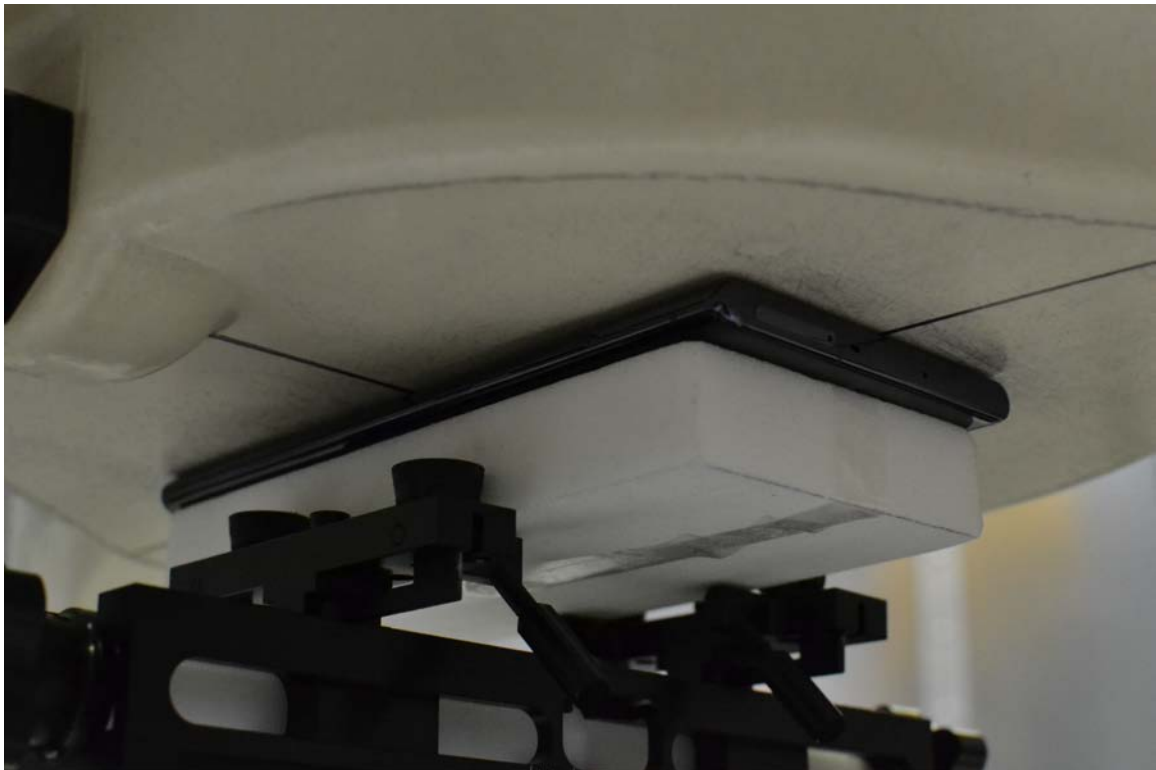
SAR Test Setup Photo 8 – Back Side at 0 mm
