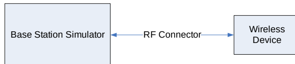
Figure 9-3 Power Measurement Setup
