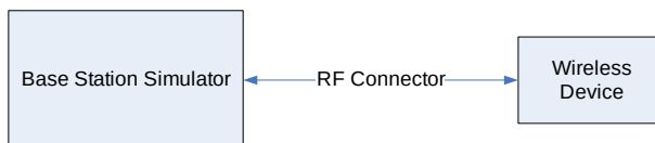
Figure 9-2 Power Measurement Setup
