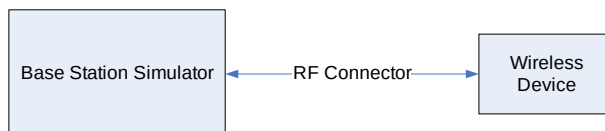
Figure 9-4 Power Measurement Setup
