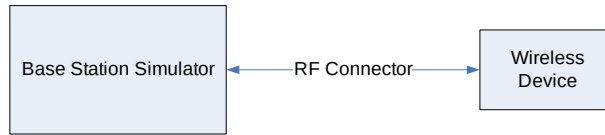
Figure 9-1 Power Measurement Setup
