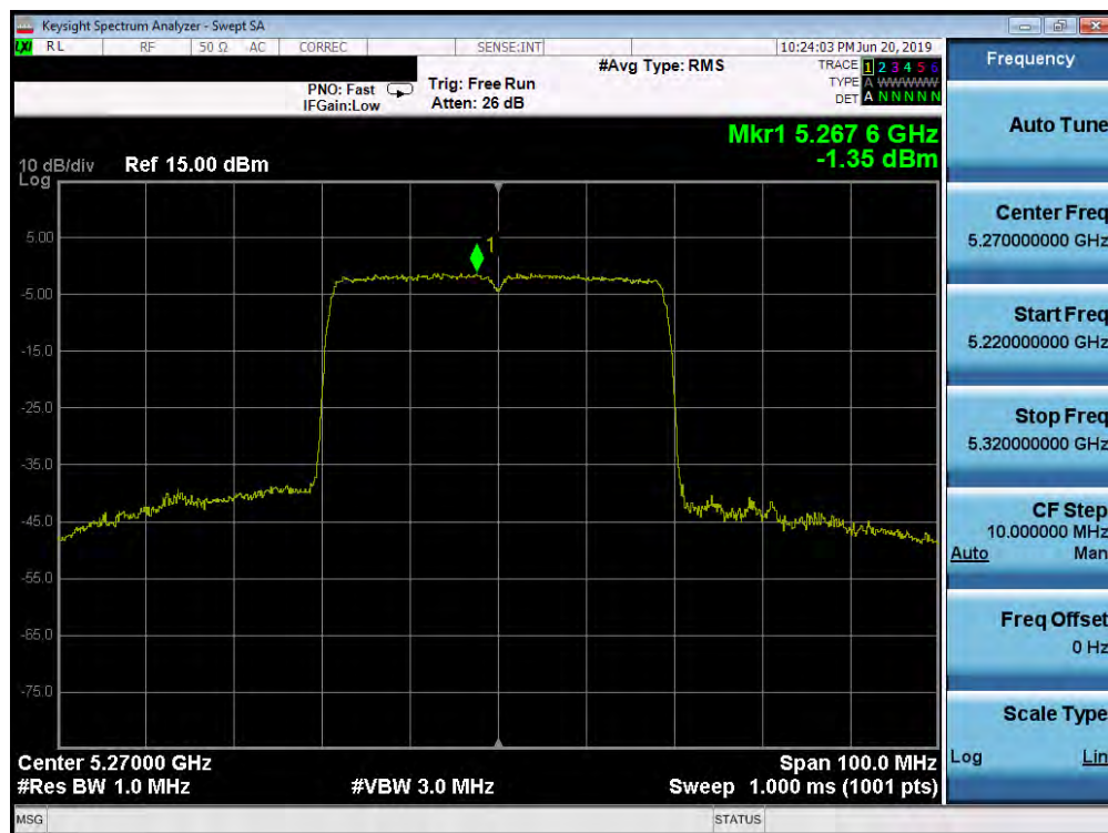
Plot 7-307. Power Spectral Density Plot MIMO ANT2 (40MHz BW 802.11ax – Full Tones (UNII Band 2A) – Ch. 54)
