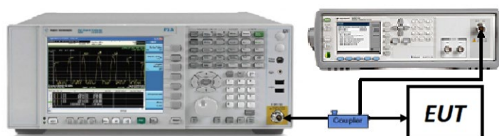
Figure 7-3. Test Instrument & Measurement Setup
