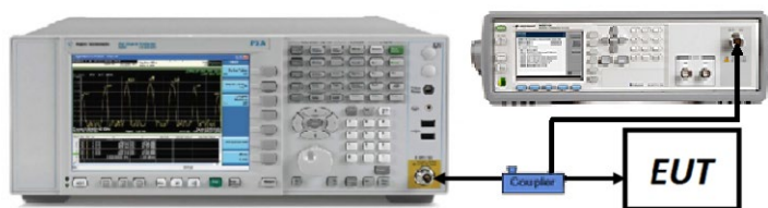
Figure 7-2. Test Instrument & Measurement Setup
