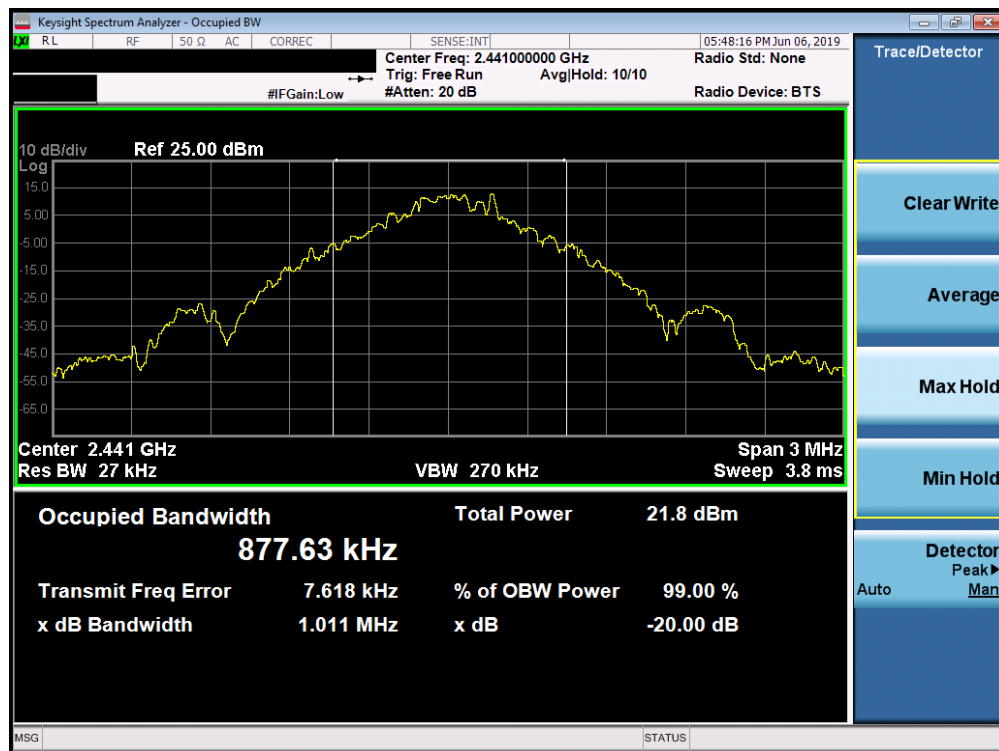
Plot 7-2. 20dB Bandwidth Plot (Bluetooth, 1Mbps – Ch. 39)
