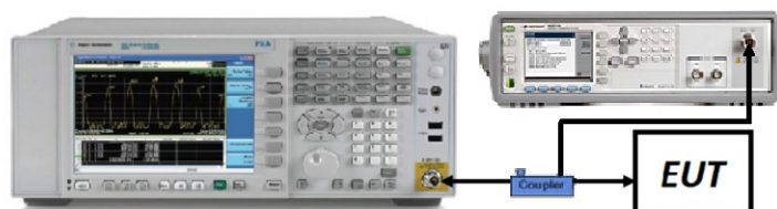
Figure 7-6. Test Instrument & Measurement Setup
