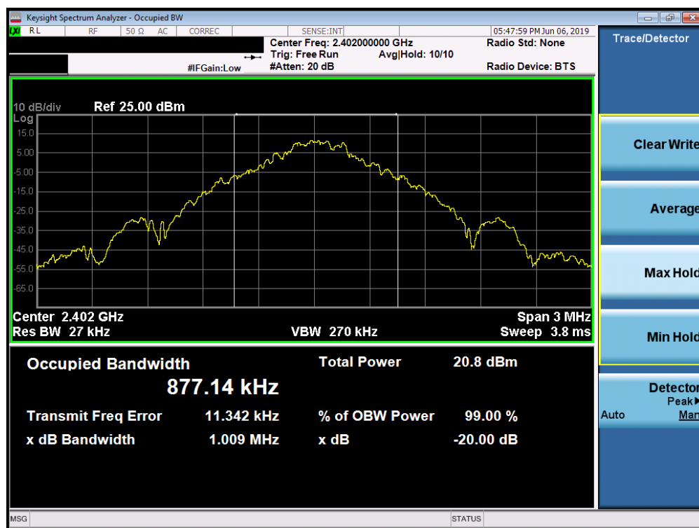
Plot 7-1. 20dB Bandwidth Plot (Bluetooth, 1Mbps – Ch. 0)
