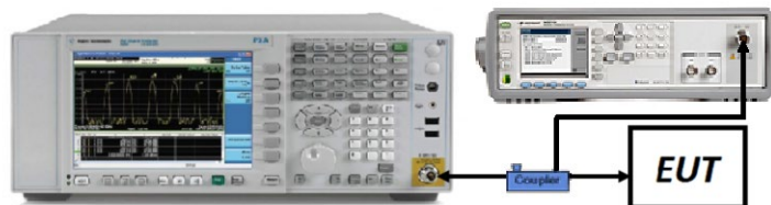
Figure 7-1. Test Instrument & Measurement Setup
