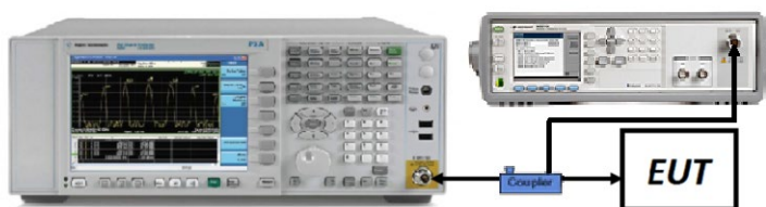
Figure 7-5. Test Instrument & Measurement Setup
