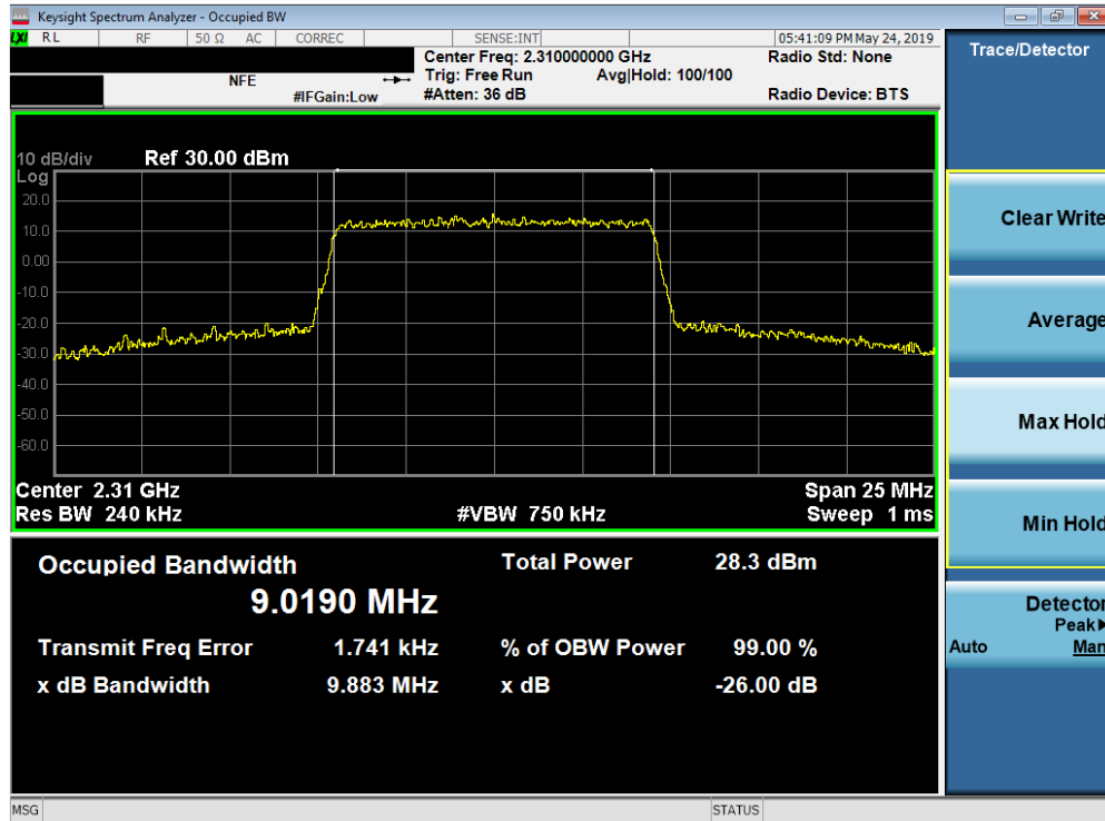
Plot 7-115. Occupied Bandwidth Plot (Band 30 - 10.0MHz 64-QAM - Full RB Configuration)
