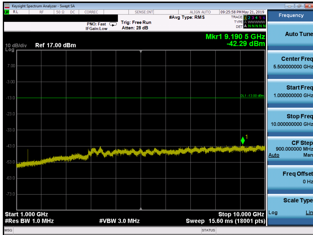
Plot 7-182. Conducted Spurious Plot (Band 12 - 10.0MHz QPSK - RB Size 1, RB Offset 0 - High Channel)
