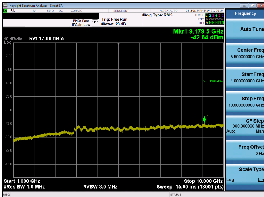
Plot 7-170. Conducted Spurious Plot (Band 71 - 20.0MHz QPSK - RB Size 1, RB Offset 0 - Mid Channel)
