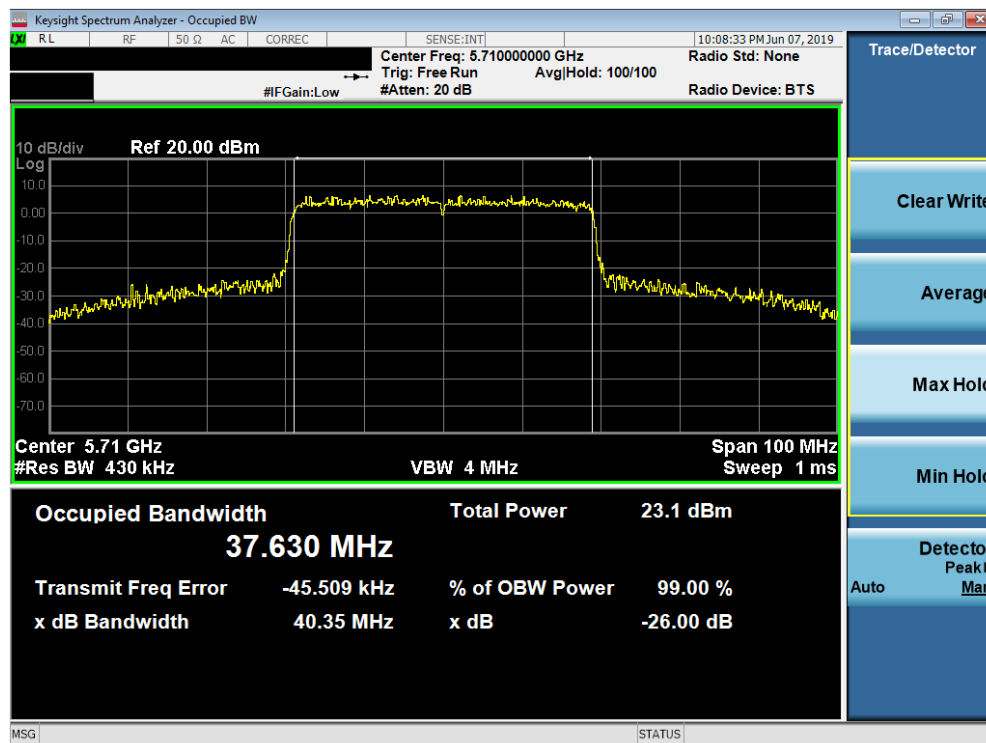
Plot 7-45. 26dB Bandwidth Plot SISO ANT1 (40MHz BW 802.11ax (UNII Band 2C) – Ch. 142)
