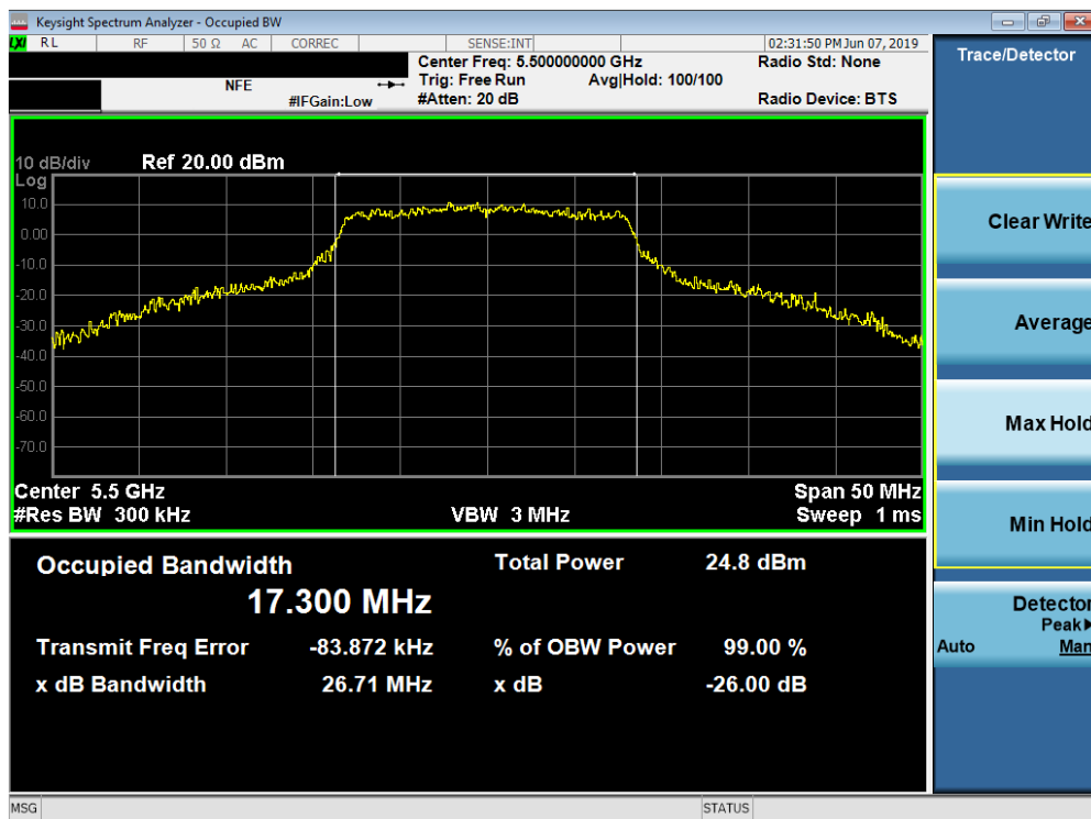
Plot 7-82. 26dB Bandwidth Plot SISO ANT2 (802.11a (UNII Band 2C) – Ch. 100)
