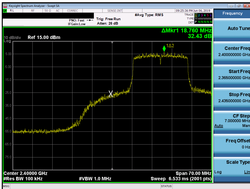
Plot 7-78. Band Edge Plot SISO ANT2 (802.11ax(2.4GHz) – Ch. 2)
