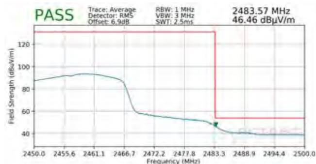
Plot 7-117. Radiated Restricted Upper Band Edge Measurement SISO ANT2 (Average)
