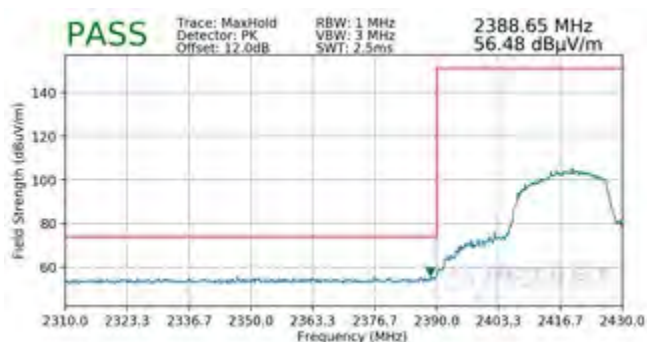
Plot 7-116. Radiated Restricted Lower Band Edge Measurement SISO ANT2 (Peak)
