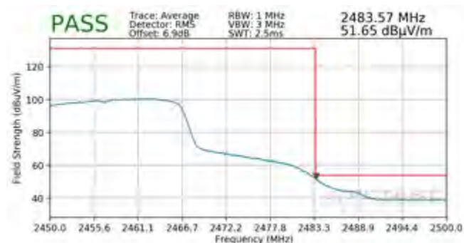
Plot 7-125. Radiated Restricted Upper Band Edge Measurement MIMO (Average)
