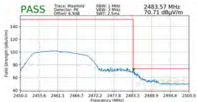
Plot 7-120. Radiated Restricted Upper Band Edge Measurement SISO ANT2 (Peak)
