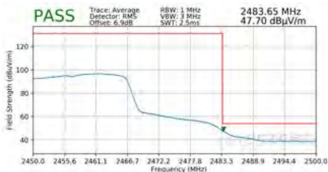
Plot 7-129. Radiated Restricted Band Edge Measurement MIMO with WCP (Average)
