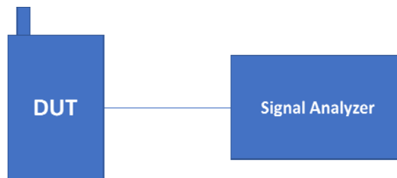
Figure 5-1 Power Measurement Setup for licensed modes
