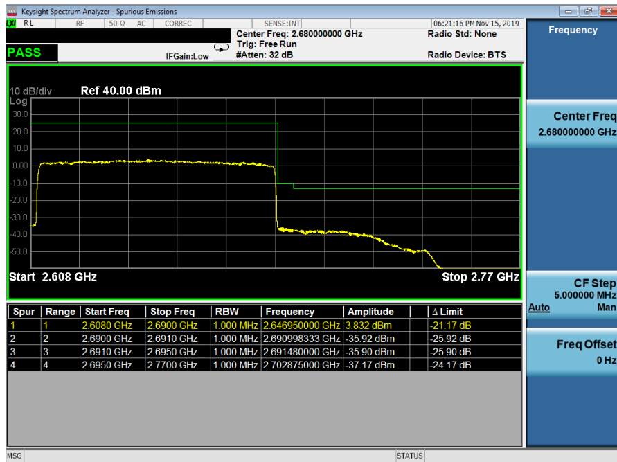
Plot 7-47. Upper ACP Plot (n41 - 80MHz DFT-QPSK - Full RB Configuration)
