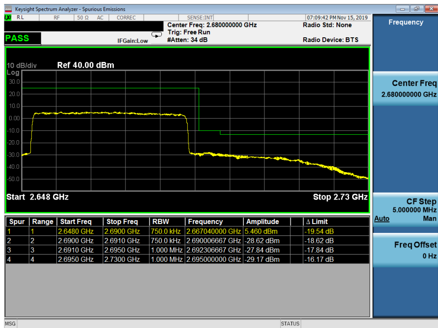
Plot 7-41. Upper ACP Plot (n41 - 40MHz DFT-QPSK - Full RB Configuration)
