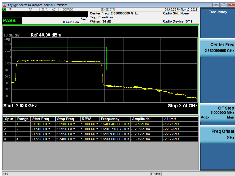
Plot 7-43. Upper ACP Plot (n41 - 50MHz DFT-QPSK - Full RB Configuration)
