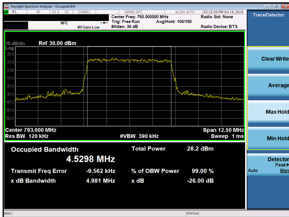
Plot 7-24. Occupied Bandwidth Plot (LTE Band 14, 5MHz 256-QAM – RB Size 25)
