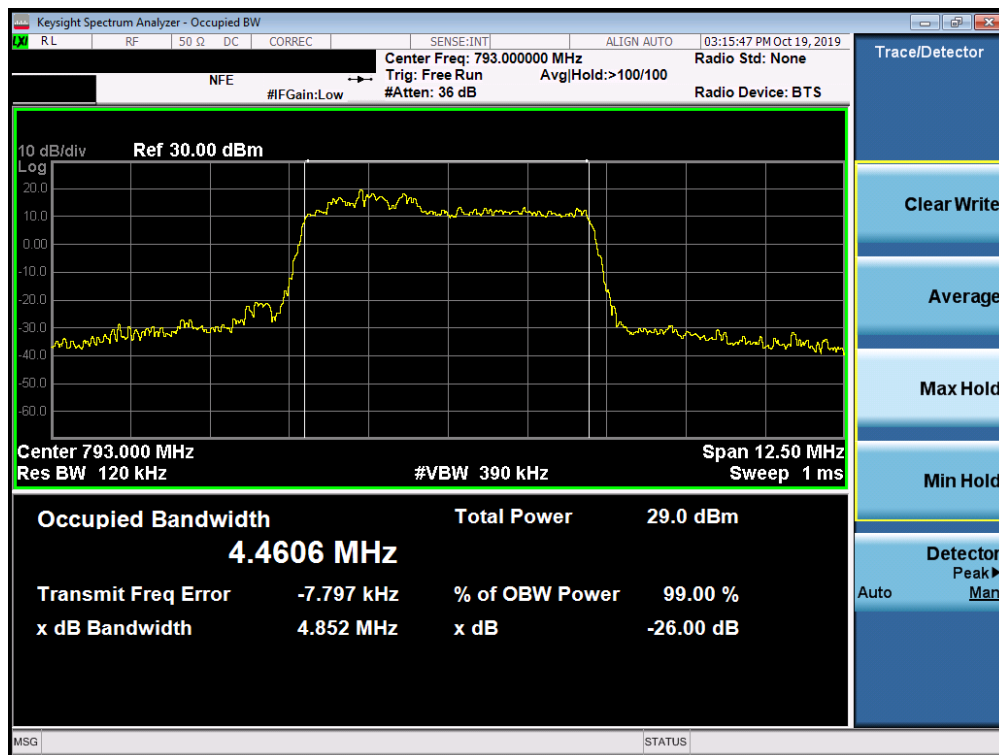
Plot 7-23. Occupied Bandwidth Plot (LTE Band 14, 5MHz 64-QAM – RB Size 25)
