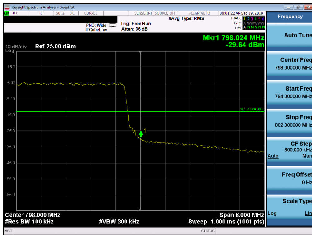
Plot 7-49. Upper Band Edge Plot (LTE Band 14, 10MHz QPSK - RB Size 50)
