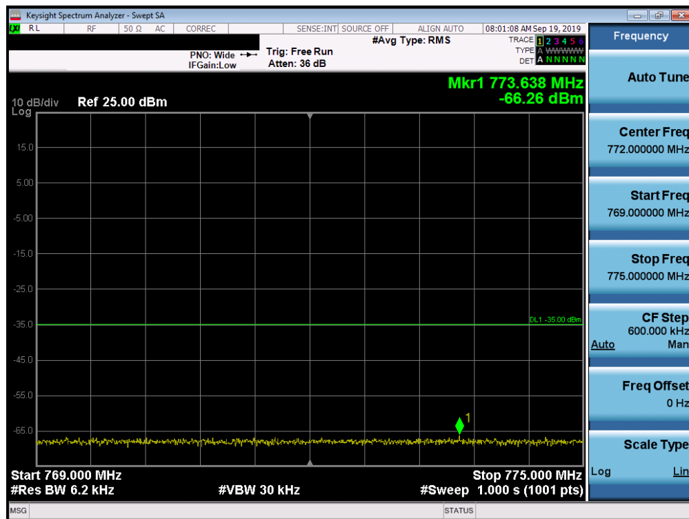
Plot 7-48. Lower Emission Mask Plot (LTE Band 14, 10MHz QPSK – RB Size 50)
