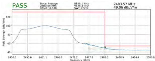
Plot 7-93. Radiated Restricted Band Edge Measurement SISO ANT1 with WCP (Average)
