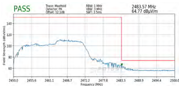
Plot 7-92. Radiated Restricted Upper Band Edge Measurement SISO ANT1 (Peak)
