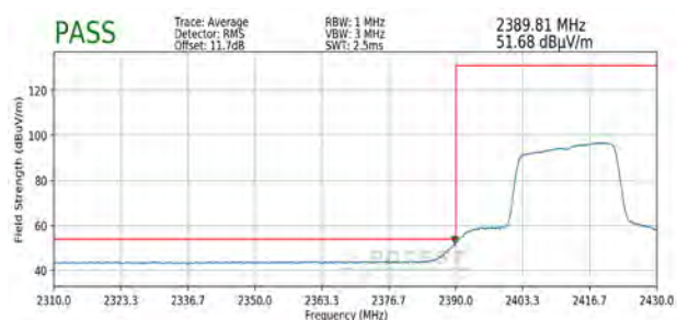
Plot 7-89. Radiated Restricted Lower Band Edge Measurement SISO ANT1 (Average)
