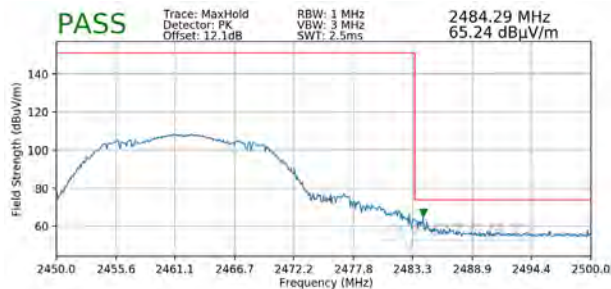
Plot 7-106. Radiated Restricted Band Edge Measurement MIMO with WCP (Peak)
