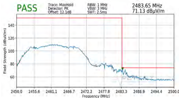
Plot 7-104. Radiated Restricted Upper Band Edge Measurement MIMO (Peak)
