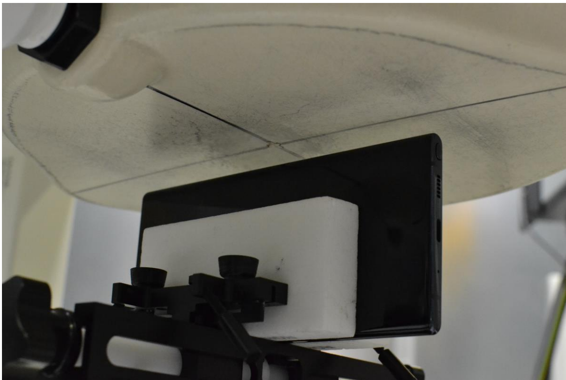
SAR Test Setup Photo 9 – Right Side at 10 mm
