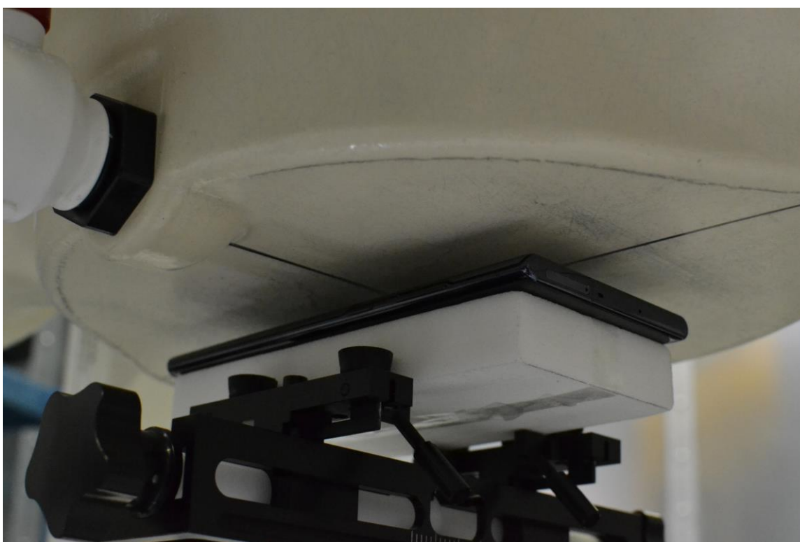
SAR Test Setup Photo 6 – Back Side at 10 mm
