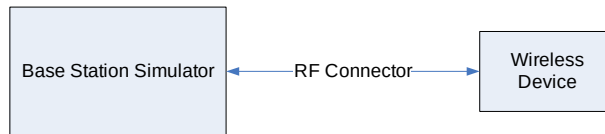
Figure 9-3 Power Measurement Setup
