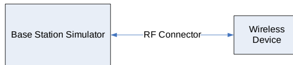
Figure 9-4 Power Measurement Setup
