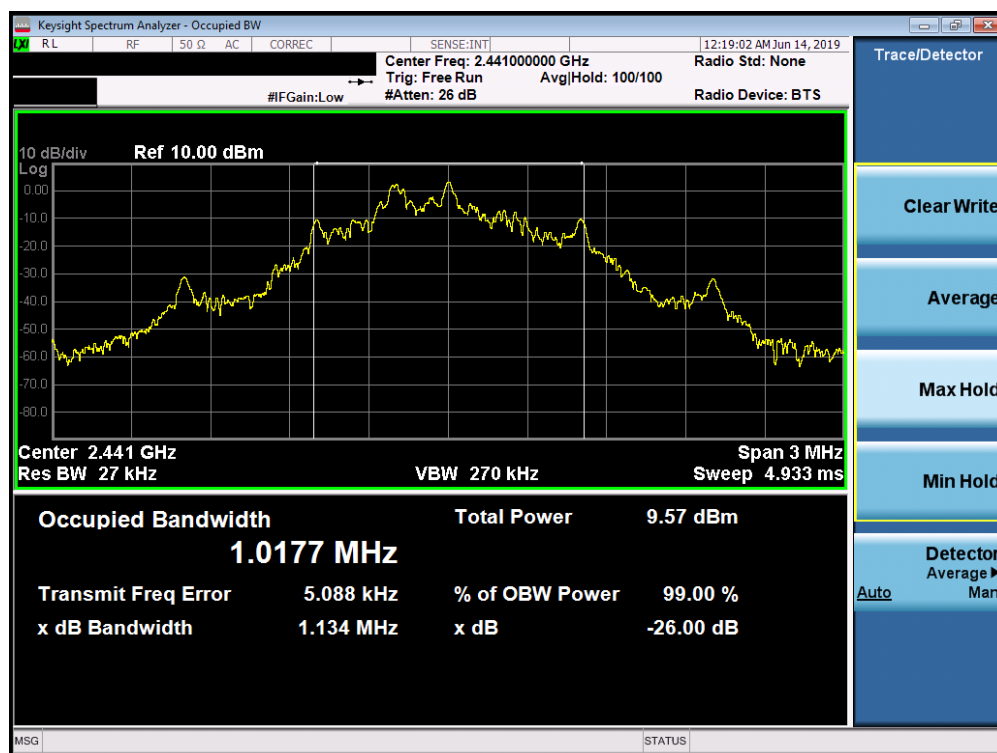
Plot 7-1. Occupied Bandwidth Plot (ANT+ – Ch. 39)
