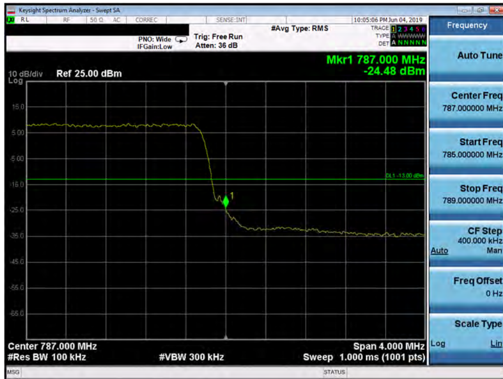
Plot 7-192. Upper Band Edge Plot (Band 13 - 5.0MHz QPSK - Full RB Configuration)
