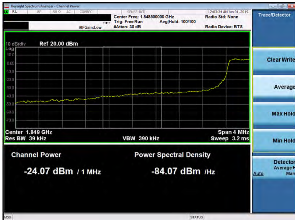
Plot 7-249. Lower Extended Band Edge Plot (Band 2 - 3.0MHz QPSK - Full RB Configuration)
