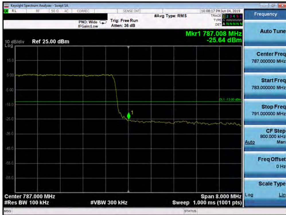
Plot 7-196. Upper Band Edge Plot (Band 13 - 10.0MHz QPSK - Full RB Configuration)
