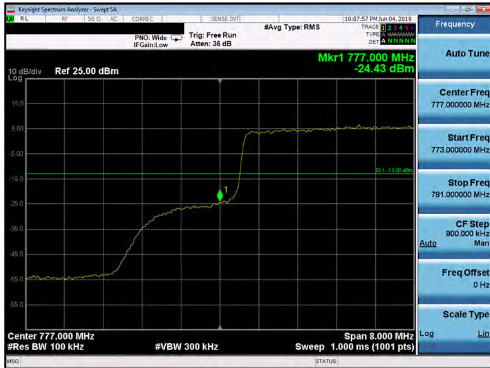
Plot 7-194. Lower Band Edge Plot (Band 13 - 10.0MHz QPSK - Full RB Configuration)
