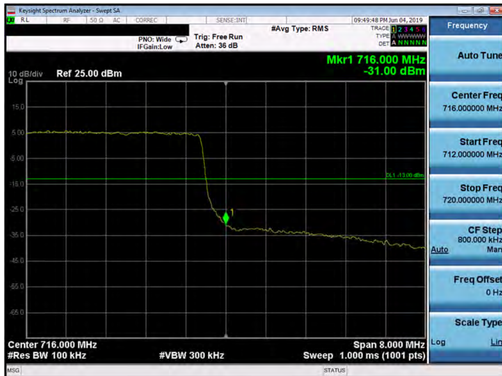
Plot 7-189. Upper Band Edge Plot (Band 12 - 10.0MHz QPSK - Full RB Configuration)
