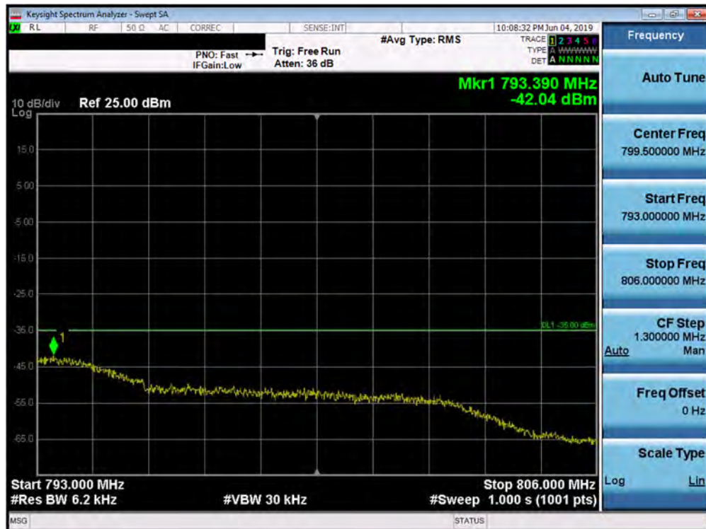
Plot 7-197. Upper Emission Mask Plot (Band 13 - 10.0MHz QPSK - Full RB Configuration)
