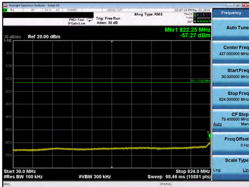
Plot 7-340. Conducted Spurious Plot (Band 5 – 10.0MHz QPSK – PCC 1/0 SCC 1/49 – High Channel)
