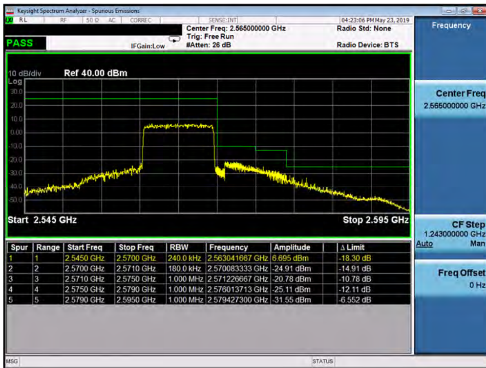
Plot 7-271. Upper ACP Plot (Band 7 - 10.0MHz QPSK - Full RB Configuration)
