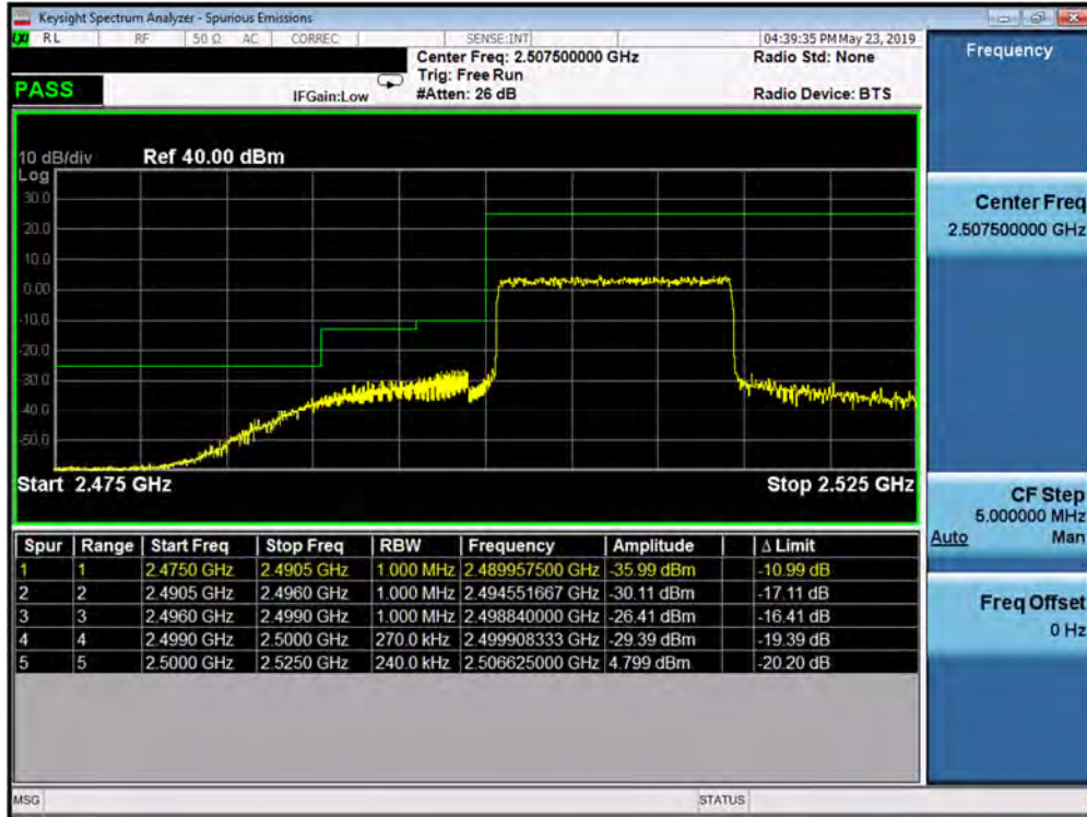
Plot 7-272. Lower ACP Plot (Band 7 - 15.0MHz QPSK - Full RB Configuration)
