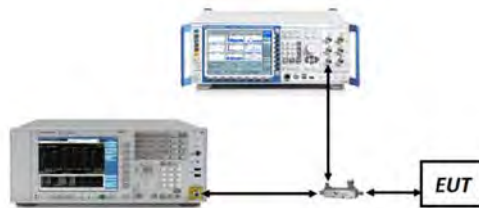
Figure 7-5. Test Instrument & Measurement Setup
