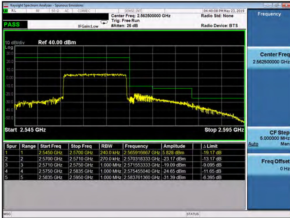
Plot 7-273. Upper ACP Plot (Band 7 - 15.0MHz QPSK - Full RB Configuration)
