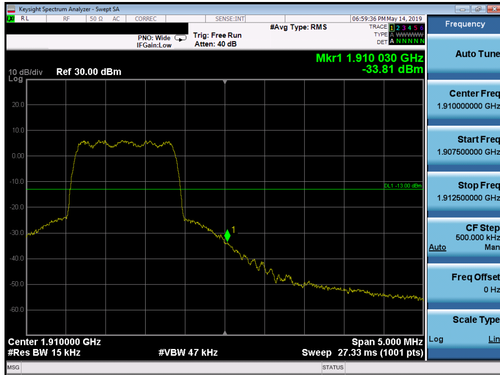
Plot 7-74. Band Edge Plot (PCS CDMA Mode - High Channel)
