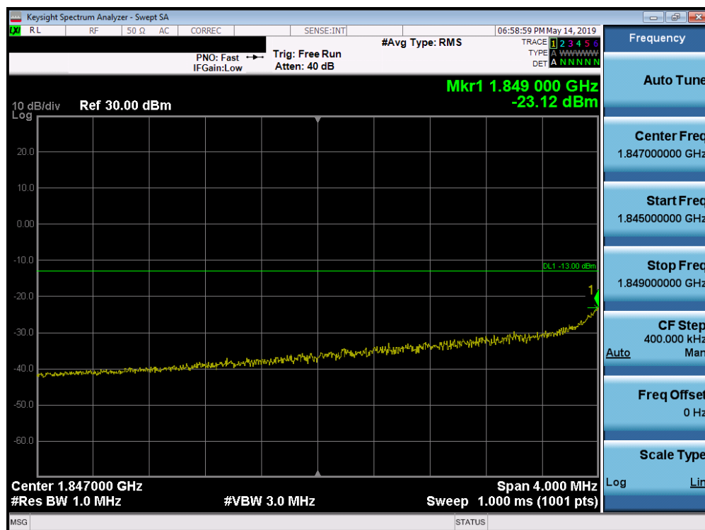
Plot 7-73. 4MHz Span Plot (PCS CDMA Mode - Low Channel)
